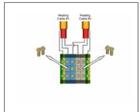
End Termination (1 to 2 Heating Cables)
