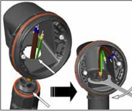
**10.** Mount junction box base on expediter. Make sure to align slots to properly orient junction box base. Tighten nut with Terminator-LN-Tool. If mounting horizontally, threaded gland holes must face downward.
