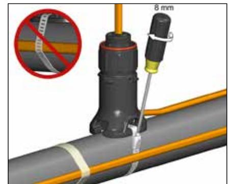
**6.** Mount expediter to pipe using pipe band. Do not band over cable.
