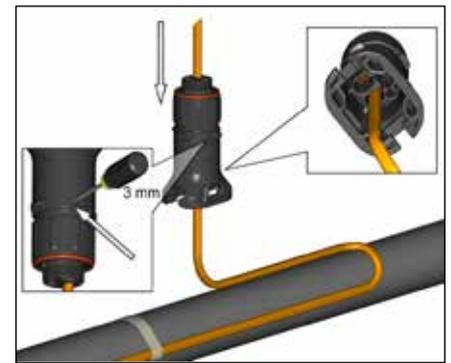
**3.** Insert cable into expediter. If mounted on bottom or side of pipe, punch out weep hole.
