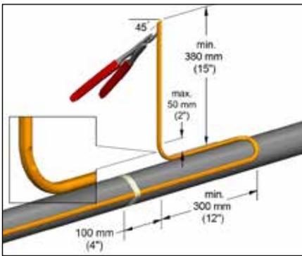
**1.** Locate bus connection (HPT and FP only) and cable as shown. Cut end of cable at angle to aid in piercing grommet. Leave additional cable for expansion loop. See page 5 for multiple cable installation tips.
