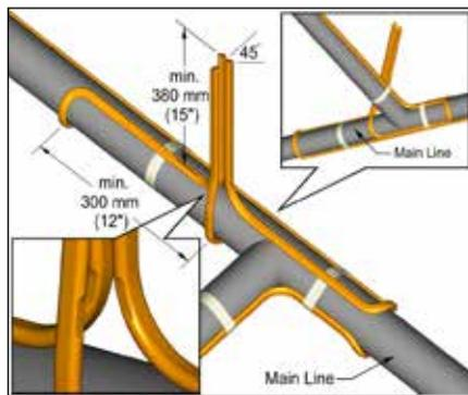
Locate bus connection (HPT and FP only) and cable as shown. Cut end of cable at angle to aid in piercing grommet. Leave additional cable for expansion loop.
