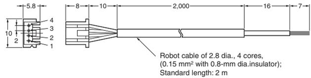
Connector with Robot Cable
