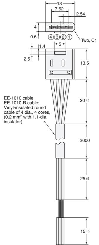
Connector with Robot Cable
