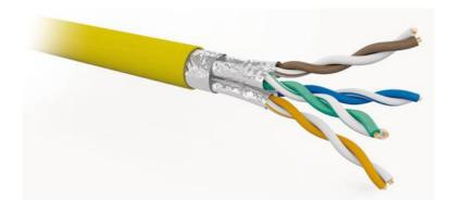
The cable has been designed to exceed the ISO/IEC, TIA and CENELEC for Category 6A/Augmented Category 6 component requirements. This delivers Class EA link performance over distances of up 90 m which supports the applications including 10GBASE-T, 10 Gigabit Ethernet.
