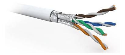
Thanks to cutting edge technoolgies, this cable is manufactured in a way to exceed the ISO, ANSI/TIA and CENELEC for Class EA, Category 6A applications. It Can easily be integrated into a Class EA link, in order to support applications up to 10GBASE-T (10Gbits Ethernet). It has a good shielding effectiveness with global and individual screened pairs (F/FTP). Compatible with all current connecting hardware in accordance with EN 50173 and ISO/IEC 11801.
