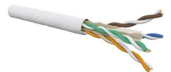
The cable has been designed to exceed the ISO/IEC, TIA and CENELEC for Category 6 component requirements. This delivers Class E link performance over distances of up 90 m which supports the applications including Gigabit Ethernet application. Small diameter cable due to specific designed cross filler
