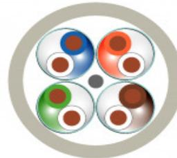
**General Construction:** Four (Dual Eight) individually foil shielded twisted pairs are cabled together into two cores. The two cores are laid in parallel and jacketed (dual in a FIG-8)
