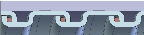
Square-Locked Design with integral bonding wire 1/2" through 1"
