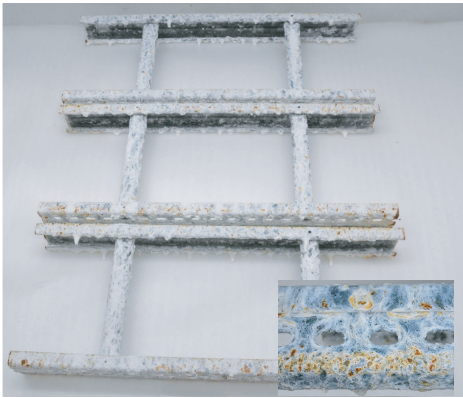
After 768 h red rust has occurred. HDG cable ladders fails after 1000 h.
