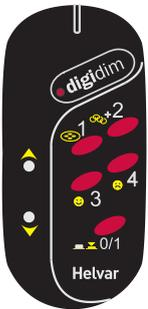
Select the operating modes by pressing the below mentioned button combination for about 10 seconds. The product confirms the successful programming by flashing the lamps
