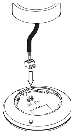
4. Re-attach the receiver housing (align with the housing mounting, insert and twist). Power on the DALI network.
