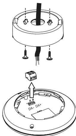
3. Connect the DALI wires and tighten the screws (the gateway is not polarity-sensitive). Re-attach the DALI connector block.
