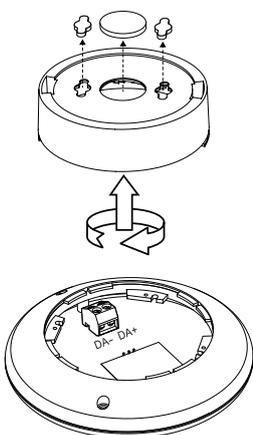
2. Thread the DALI cable through the housing mounting, and screw the housing mounting in place. Remove the DALI connector block from the receiver housing.
