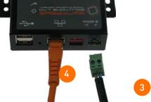
The BACnet Gateway is typically installed as part of a control system using an Ethernet hub/switch. Category 5 cables can be used for individual line lengths of up to 100 metres.
