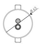
When placing unit into assembly hole (Ø 50-55mm) ensure locking springs are in this position.
