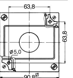
The fixing holes (diam. 5,0 mm) can be accessed after removing the cover (4 screws). Warning: the photocell opening should not be reached by the light controlled by the twilight switch.
