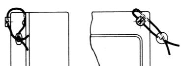
1. Remove the top right cover screw and replace it with the seal screw supplied which has a transverse hole.
