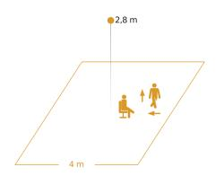
Possible mounting height: 2,50 m – 4,00 m Orange: presence, tangential and radial
