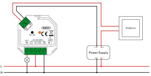
This phase dimmer adopts trailing edge dimming (reverse phase control), please make sure the connected loads support reverse phase control. Please refer to the user manual of the load or consult the supplier of the load.
