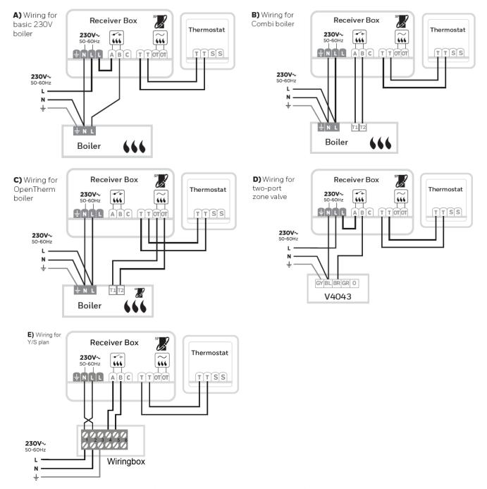
Note: Wiring diagrams are for Lyric T6 wired thermostat solution, for Lyric T6R wireless thermostat the thermostat is not wired to the Receiver box and the terminals are also not available.
