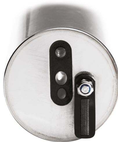
Figure 3 Auto-clean system overcomes optical fouling
