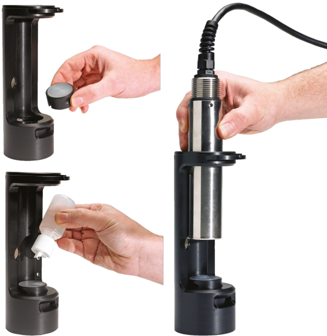
Figure 6 ATS430 easy calibration procedure
