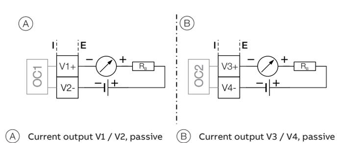
Figure 44: (I = internal, E = external, RB = load)
