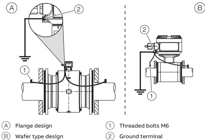
Figure 30: Metal pipe, without liner (example)
