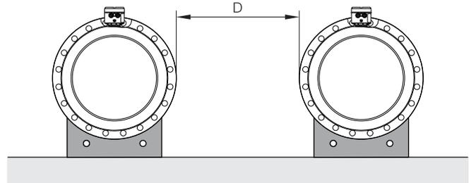
Spacing D:  $\geq 1.0$  m (3.3 ft) for Design Level 'A',
