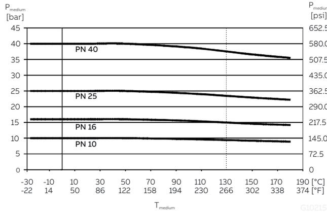
Figure 81: DIN flange, stainless steel, up to DN 100 (4 in)
