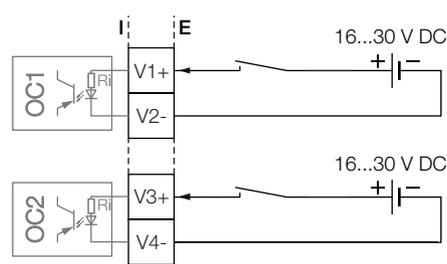
Figure 47: Plug-in card as digital input (I = internal, E = external)
