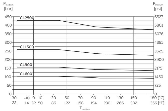
Figure 77: ASME flange, steel, DN 25 to 400 (1 to 24 in); Design Level 'A'
