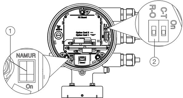
① NAMUR DIP switch                      ② Write protection DIP switch
