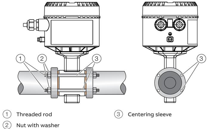
Figure 6: Assembly set for wafer type assembly (example)
