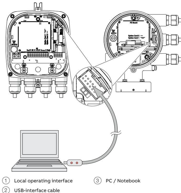
Figure 66: Connection to the local operating interface
