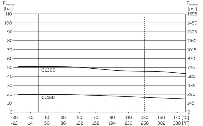
**Figure 74: ASME-flange, steel up to DN 400 (16 in) (CL150/300) to DN 1000 (40 in) (CL150); Design Level 'A'**
