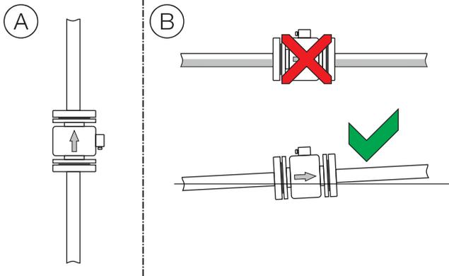
Figure 9: Mounting position
