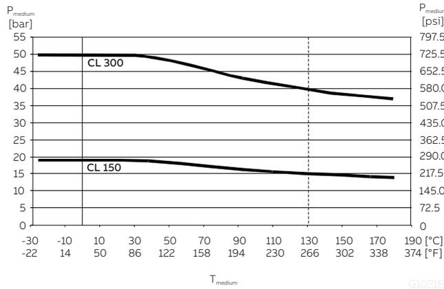
Figure 82: DIN flange, stainless steel, up to DN 100 (4 in) (CL 150 / 300)
