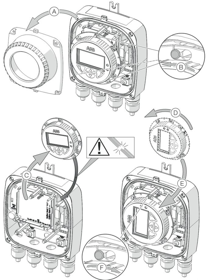
Figure 26: Rotating the LCD indicator
