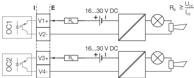
Figure 46: Plug-in card as binary output (I = internal, E = external,  $R_B$  = load)
