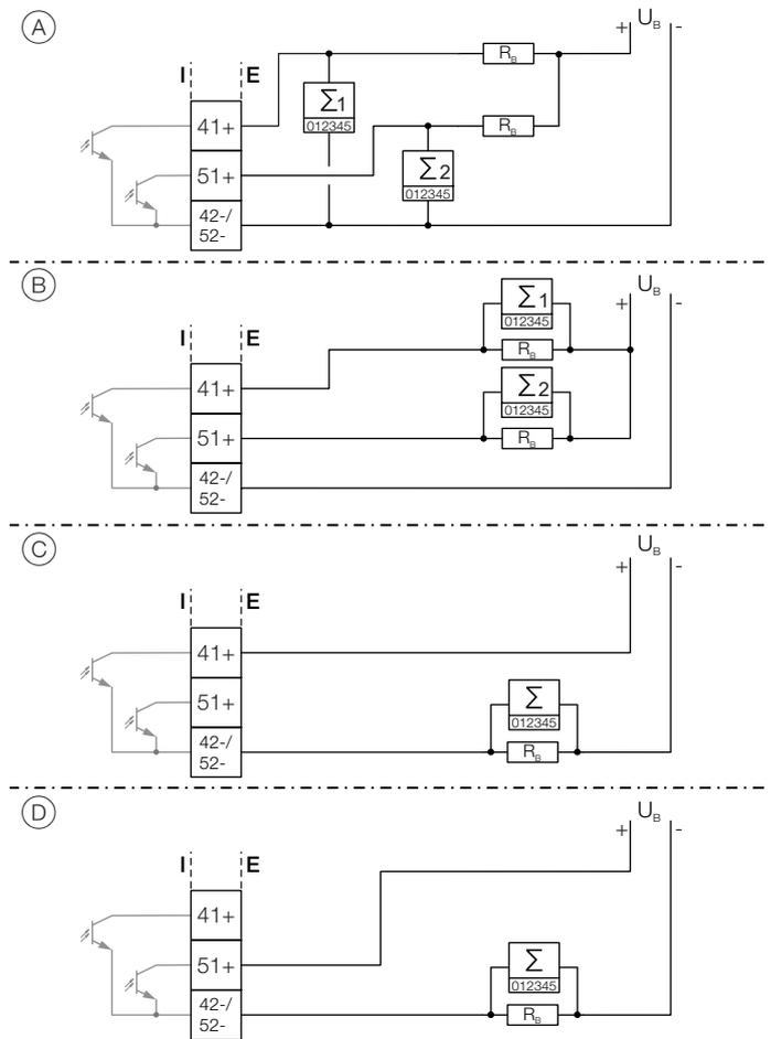
Figure 55: Connection versions digital output 41 / 42 and 51 / 52
