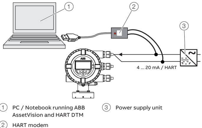
Figure 68: HART Modem on the transmitter (example)
