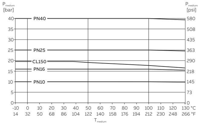
**Figure 79: Cast iron housing, DN 25 to 600 (1 to 24 in); Design Level 'B'**
