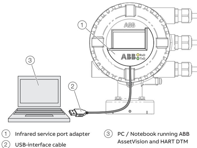
Figure 67: Infrared service port adapter on the transmitter (example)
