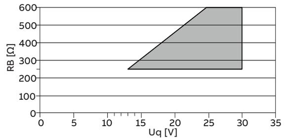
Figure 45: Source voltage for passive outputs
