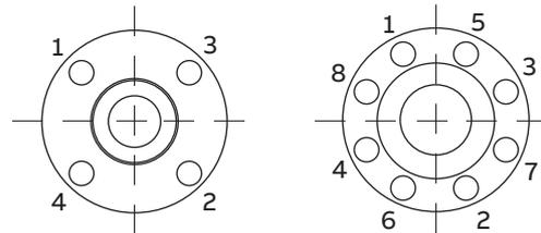
Figure 19: Tightening sequence for the flange screws
