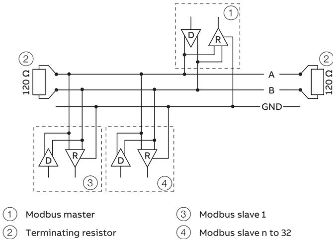
Figure 60: Communication with the Modbus protocol
