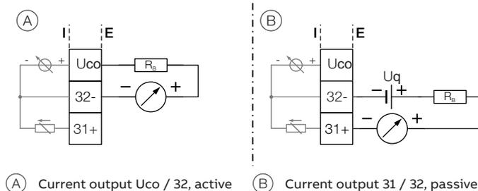
Figure 41: (I = internal, E = external,  $R_B$  = load)
