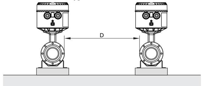
Spacing D:  $\geq 1.0$  m ( $\geq 3.3$  ft)
