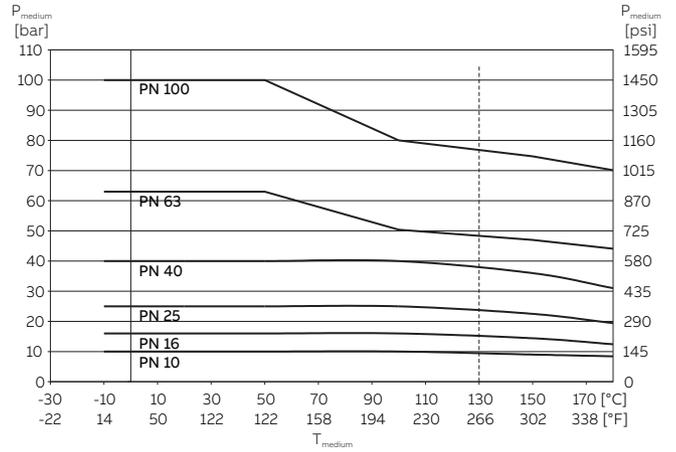
**Figure 73: DIN flange, steel up to DN 600 (24 in); Design Level 'A'**
