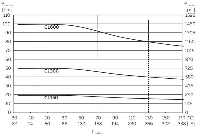
**Figure 72: ASME-flange, stainless steel, to DN 400 (16 in) (CL150/300) to DN 1000 (40 in) (CL150); Design Level 'A'**
