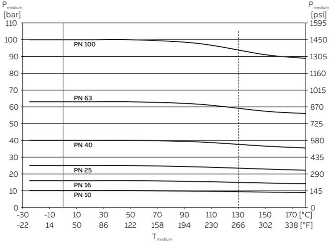
**Figure 71: DIN-flange, stainless steel, to DN 600 (24 in); Design Level 'A'**
