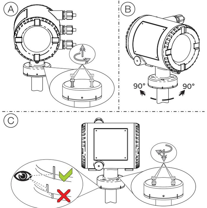
Figure 24: Rotate transmitter housing
