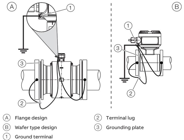
Figure 31: Plastic pipes, non-metallic pipes or pipes with insulating liner
