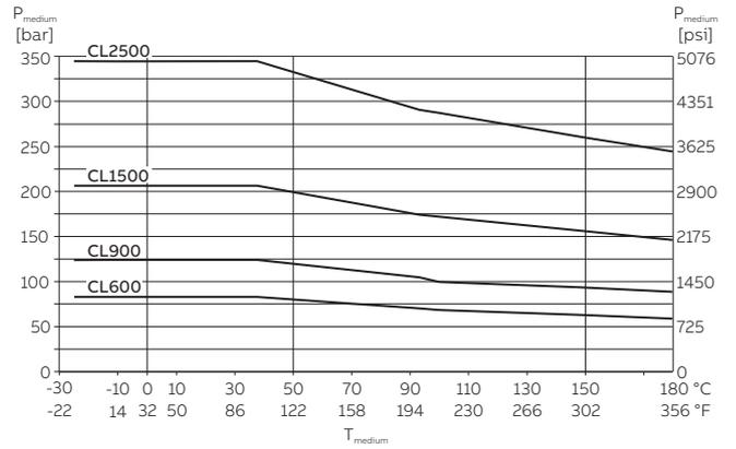
Figure 78: ASME flange, stainless steel, DN 25 to 400 (1 to 24 in); Design Level 'A'
