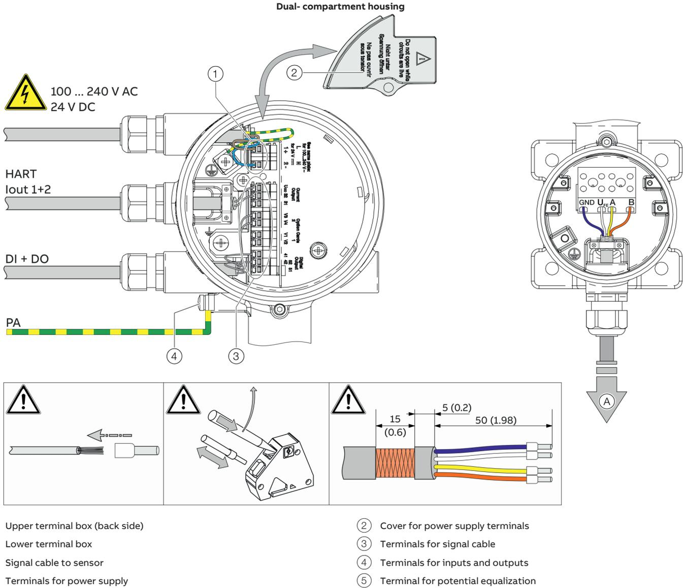
Figure 57: Electrical connection to transmitter in remote mount design [example, dimensions in mm (in)]
