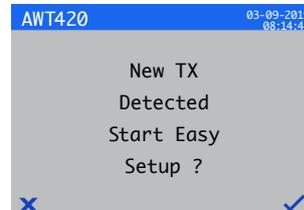
Press the key () to start Easy Setup or press the key () to cancel and exit to the main Operator page.
