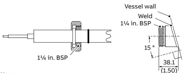
**Note.** Customer-supplied holder nut slides over sensor and threads onto tank bushing
