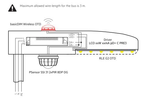
The basicDIM Wireless OTD supports the Zhaga connectivity standard for Plug&Play luminaire extensions. This allows a toolless and flexible integration in luminaires.
