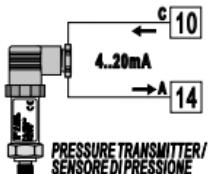
For linear signals 0/4..20 mA with two-wire sensor.
