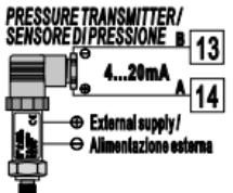
For linear signals 0/4..20 mA with external power of sensor.
