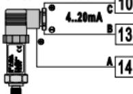
For linear signals 0/4..20 mA with three-wire sensor.
