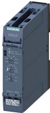
analog adjustment monitoring relay phase failure, phase sequence, asymmetry and under-voltage monitoring 3x 160-690 V AC, 15-70 Hz 2 changeover contacts screw terminal
