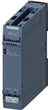
monitoring relay phase failure, phase sequence and asymmetry monitoring 3x 160-690 V AC, 15-70 Hz 2 changeover contacts screw terminal
