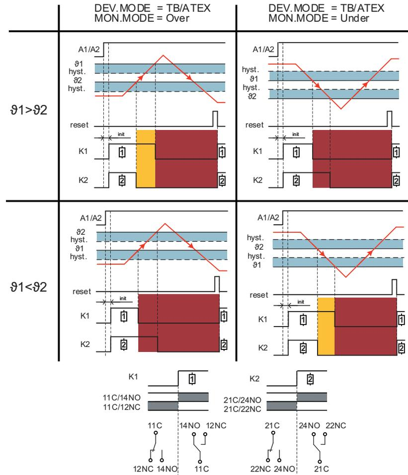
Figure 5-10 Temperature limiter time diagram TB + ATEX
