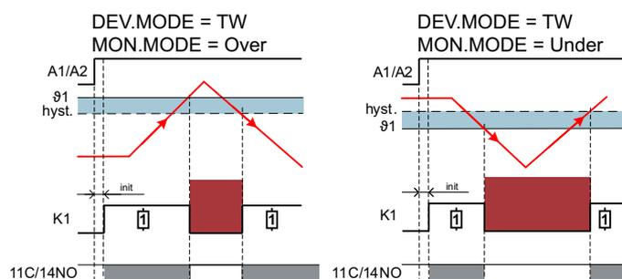
Figure 5-6 Temperature monitor safety function time diagram
