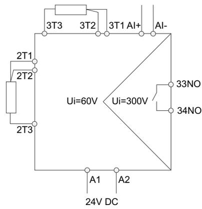
Figure 13-5 Isolation circuit diagram 3RS2900-.AA30
