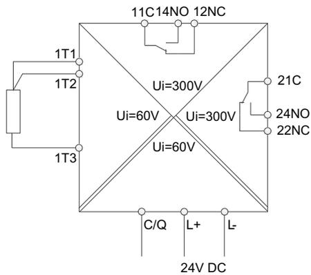
Figure 13-3 Isolation circuit diagram 3RS2800
