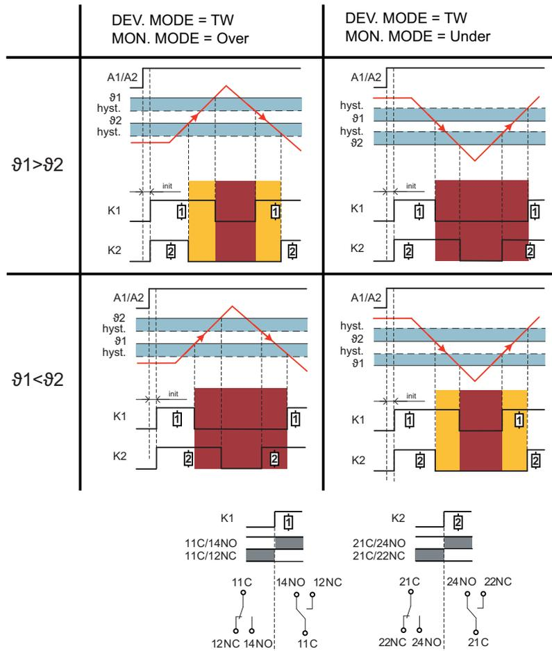
Figure 5-5 Temperature monitor time diagram
