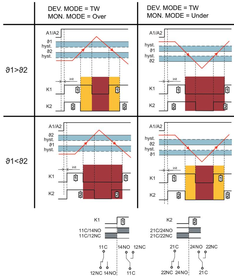
Figure 6-1 Temperature monitor time diagram TW
