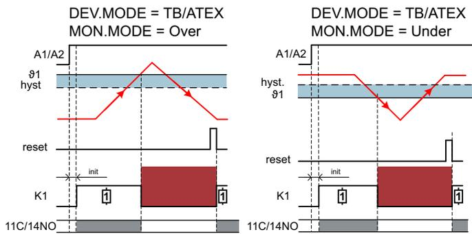
Figure 5-2 Temperature limiter safety function
