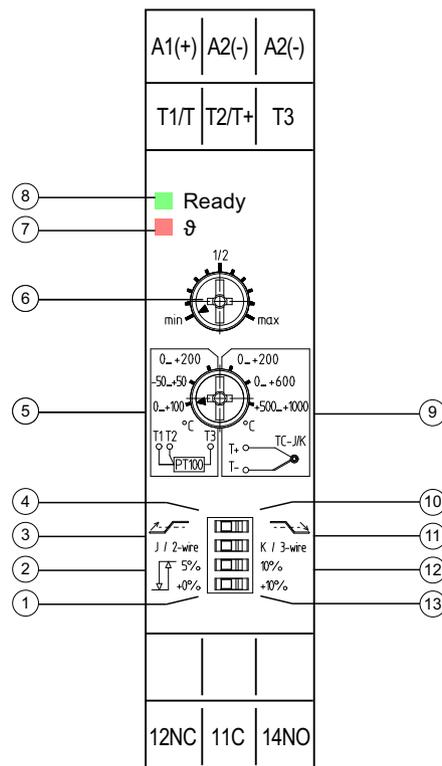
Figure 4-1 Operator controls and display elements of the analog devices
