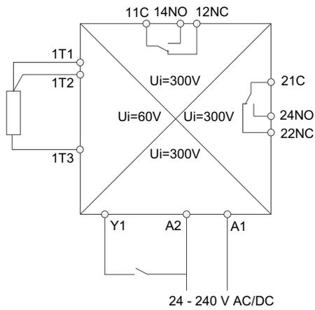
Figure 13-1 Isolation circuit diagram 3RS2600-.BW30
