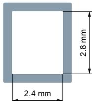
Take note of the orientation of the terminal space, which may require vertical fitting of rectangular-crimped conductors.
