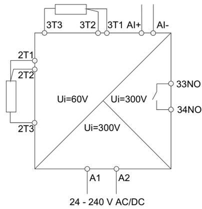
Figure 13-4 Isolation circuit diagram 3RS2900-.AW30
