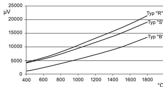
Figure 8-2 Thermocouples S, R, B
