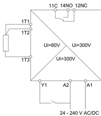
Figure 13-6 Isolation circuit diagram 3RS2500-..W..
