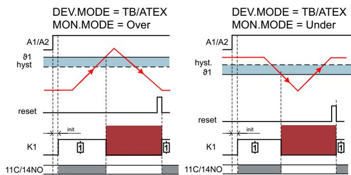
Figure 5-4 Temperature limiter safety function time diagram
