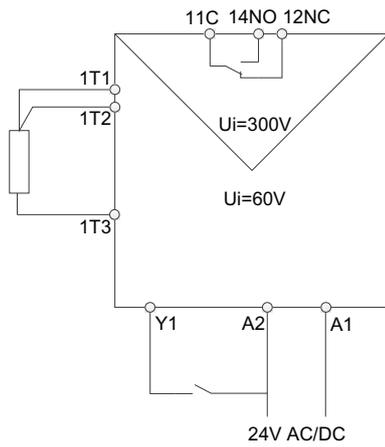
Figure 13-7 Isolation circuit diagram 3RS2500-..A..
