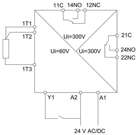
Figure 13-2 Isolation circuit diagram 3RS2600-.BA30
