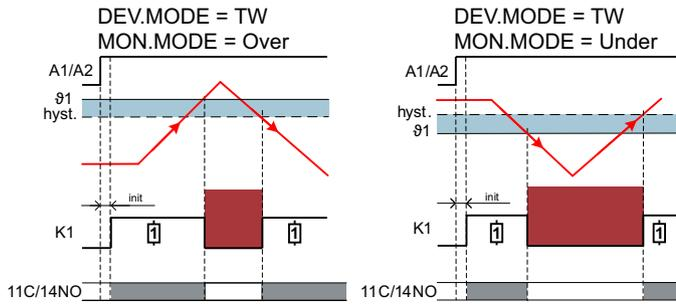
Figure 5-1 Safety function temperature monitor
