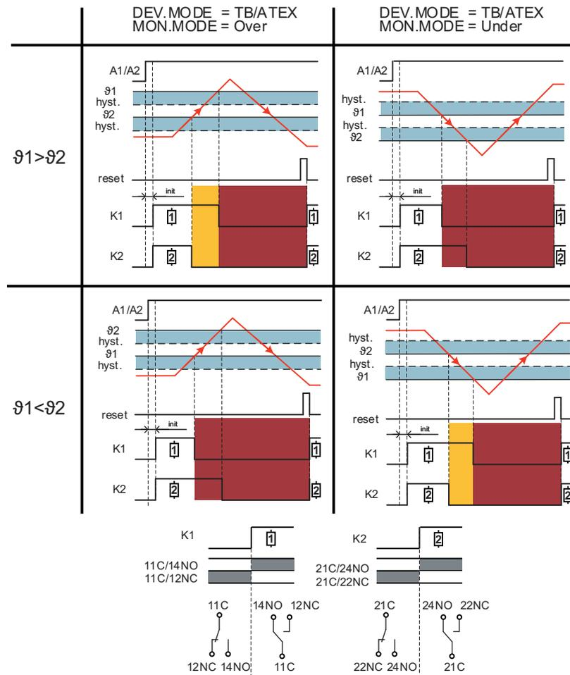
Figure 5-3 Temperature limiter time diagram
