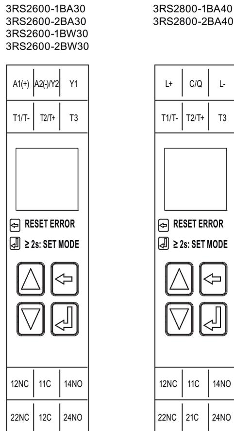
Figure 5-7 Operator controls and display elements of the digital devices
