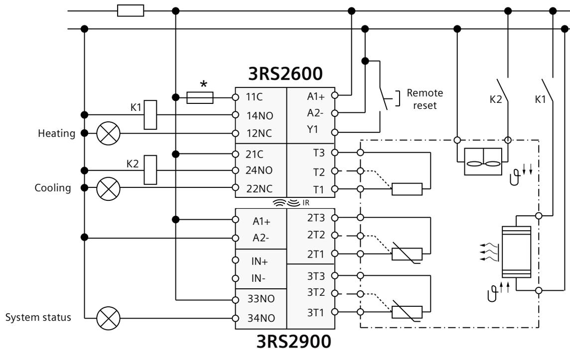
Figure 10-3 Three-step control (here with sensor expansion module)
