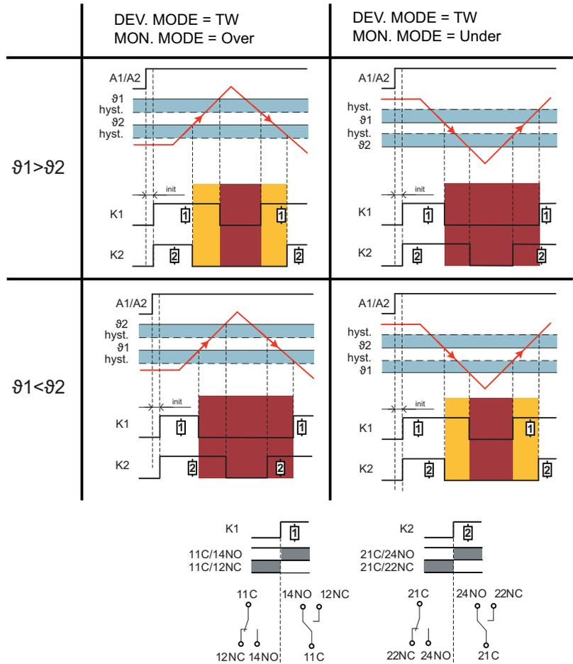
Figure 5-9 Temperature monitor time diagram TW
