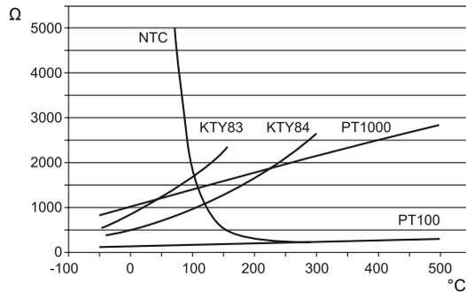
Figure 9-1 Temperature ranges of the resistance sensors
