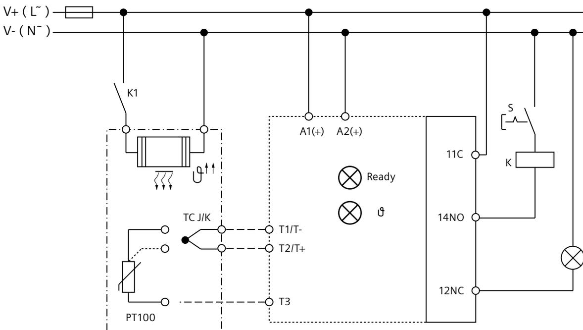
Figure 10-1 Simple two-step heating control
