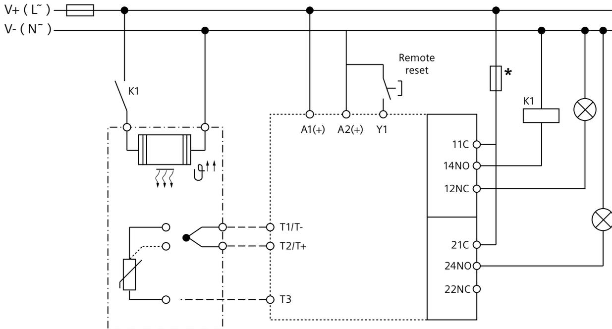
Figure 10-2 Two-step control (here with sensor expansion module)
