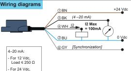
4...20 mA Sensor type Rated supply voltage Min = 9 Vdc Max = 32 Vdc with reverse polarity protection
