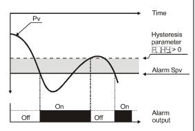
Absolute alarm with controller in cooling functioning (Par.11 Hall selected and hysteresis value greater than "0" (Par.28 HHH) > 0).
