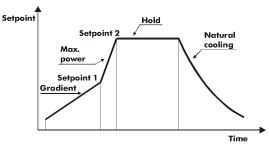
The cycle starts at each activation of the controller, or via digital input if it is enabled for this type of functioning (see parameter 61 .).
