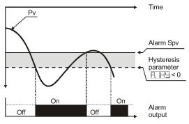
Absolute alarm with controller in cooling functioning (Par.11 日上上 selected □□□□□) and hysteresis value less than "0" (Par.28 日 田里 < 0).
