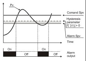
Lower deviation alarm <u>value of alarm setpoint greater than "0"</u> and <u>hysteresis value greater than "0"</u> (Par.28 | H | > 0).
