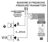
For signals 0/4....20mA with external power of sensor
