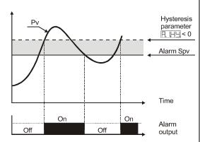
Absolute alarm with controller in heating functioning (Par.11 Hele selected Here) and hysteresis value less than "0" (Par.28 Hele < 0).
