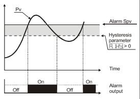
Absolute alarm with controller in heating functioning (Par.11 Hall selected HERE) and hysteresis value greater than "0" (Par.28 HH > 0).
