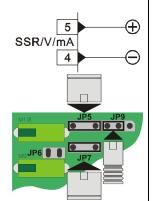
Linear output in <u>Volt</u> configurable using parameters as command (Parameter or retransmission of process-setpoint (Parameter )
