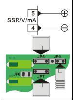
Linear output in <u>mA</u> configurable using parameters as command (Parameter cont ) or retransmission of process-setpoint (Parameter cont )
