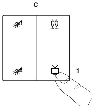
Figure 28: Saving new scene parameters
