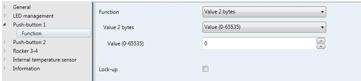
Figure 22: Function of the "Value 2 bytes" independent push-button
