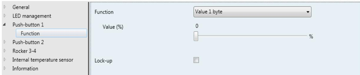
Figure 21: Function of the "Value 1 byte" rocker
