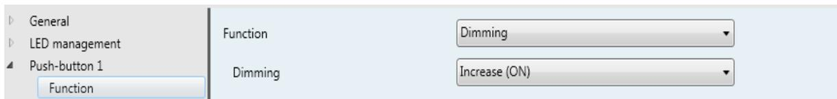
Figure 15: "Dimming" Function
