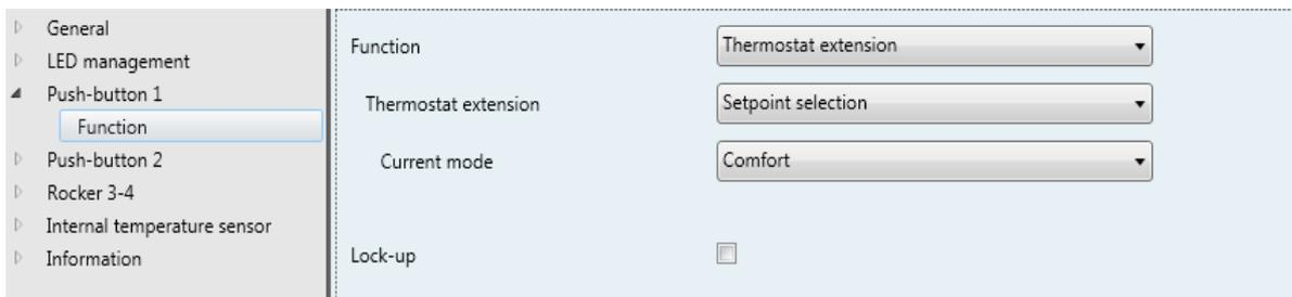
Figure 23: Function of the "Thermostat extension" independent push-button
