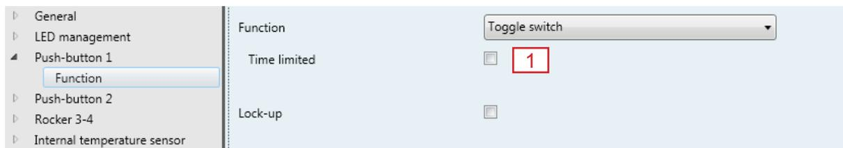
Figure 13: "Toggle switch" function of the push-button(s)
