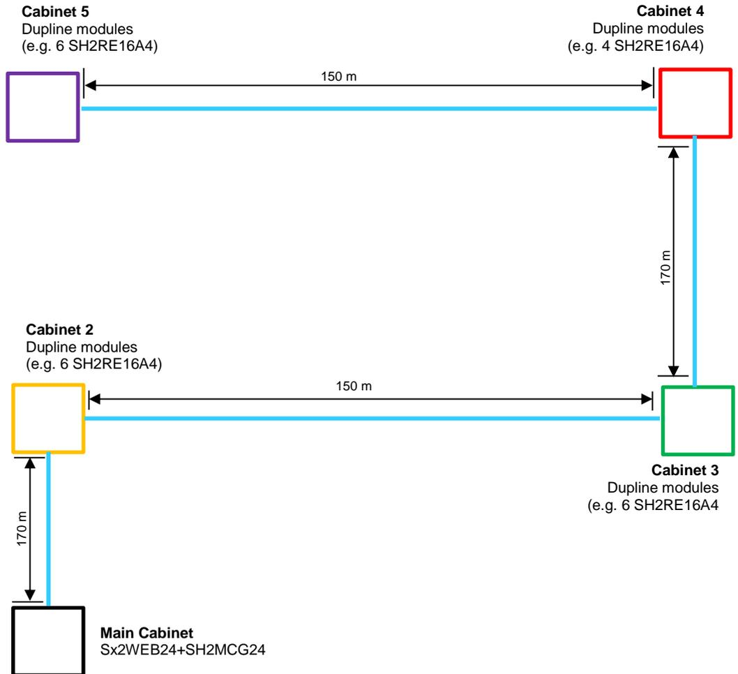
This network design is not recommended because the cable resistance and the load from bus-powered modules result in an excess of voltage drop.
