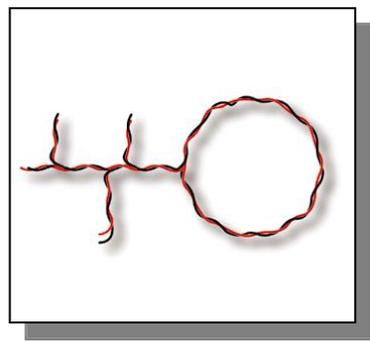
*Combined:* the best location for the SH2MCG24 is in the middle between the two farthest distant modules.
