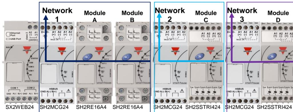
Modules **A** and **B** are connected to the Dupline® network 1.
