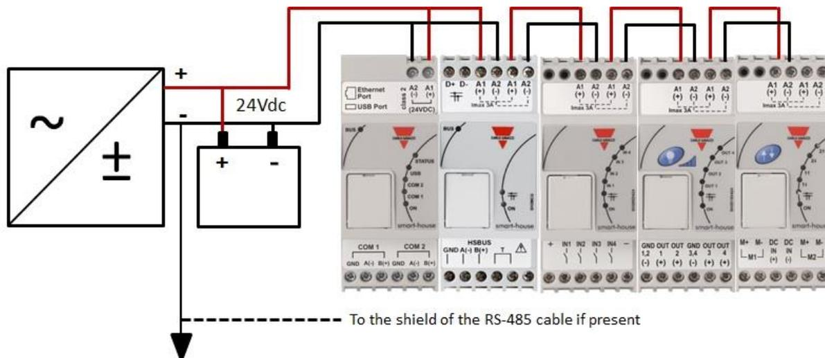
All the DIN-rail modules with the in/out terminals come with two short wires already screwed into the A1 and A2 terminals in order to speed up commissioning.
