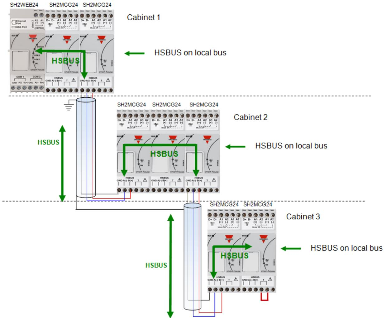
Example 3: The bus generators SH2MCG24 do not need to be put all together in a DIN rail, and they can be mixed with the Dupline® modules as is shown in the picture below.
