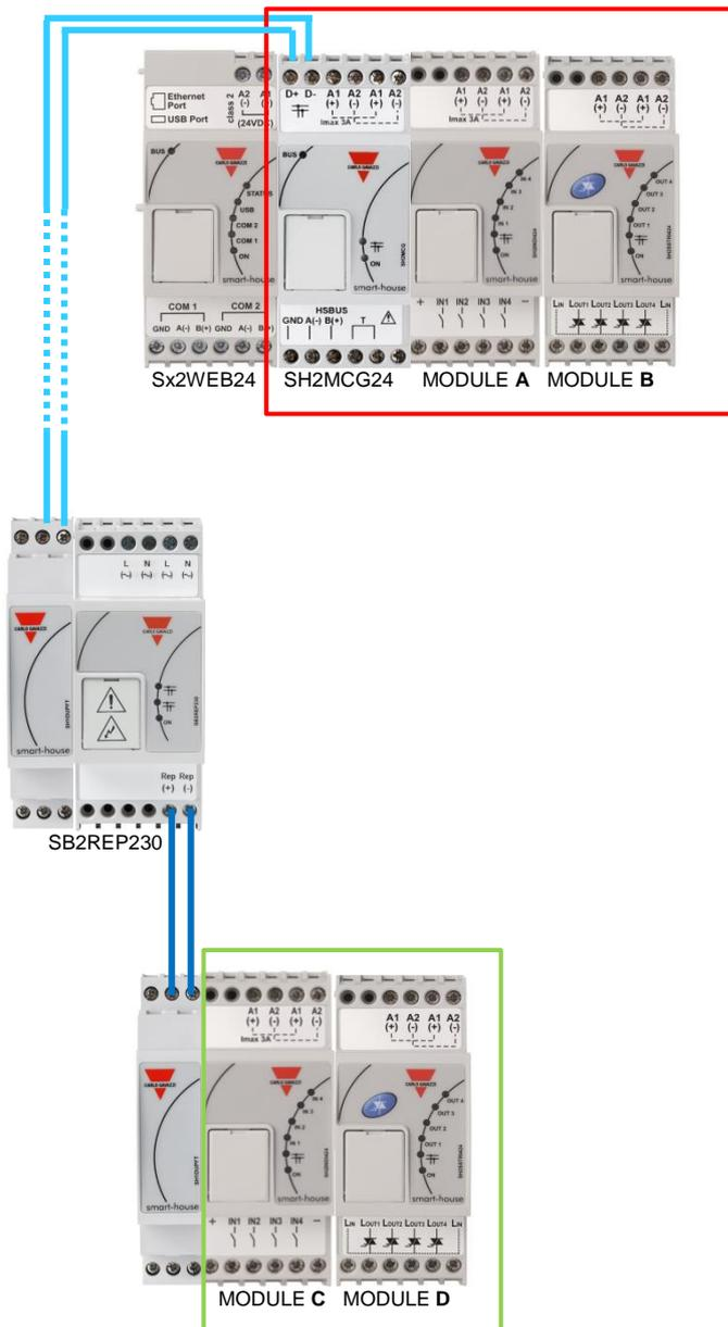
**Note:** the local bus on both sides is connected to the primary side of the Dupline network, so the secondary side has always to be connected to the terminals REP+ and REP-
