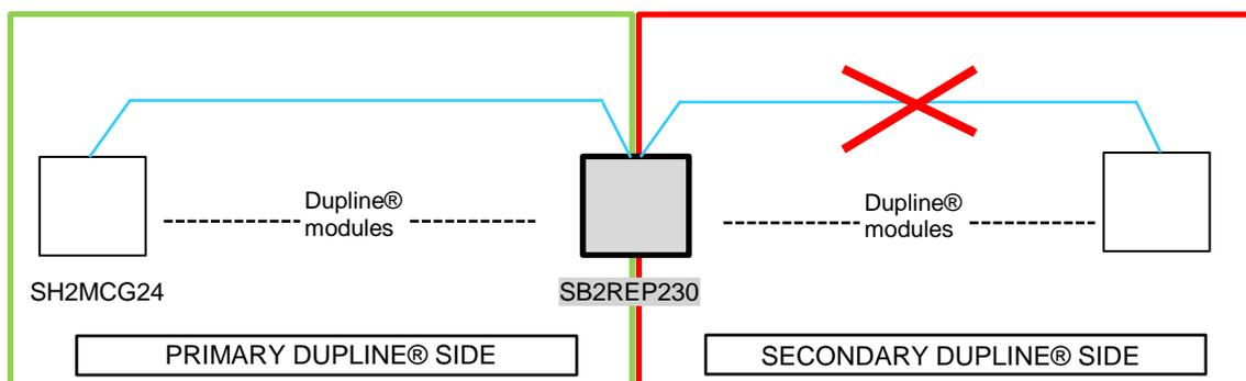
As soon as the short circuit is removed, the secondary side will automatically become operational again.
