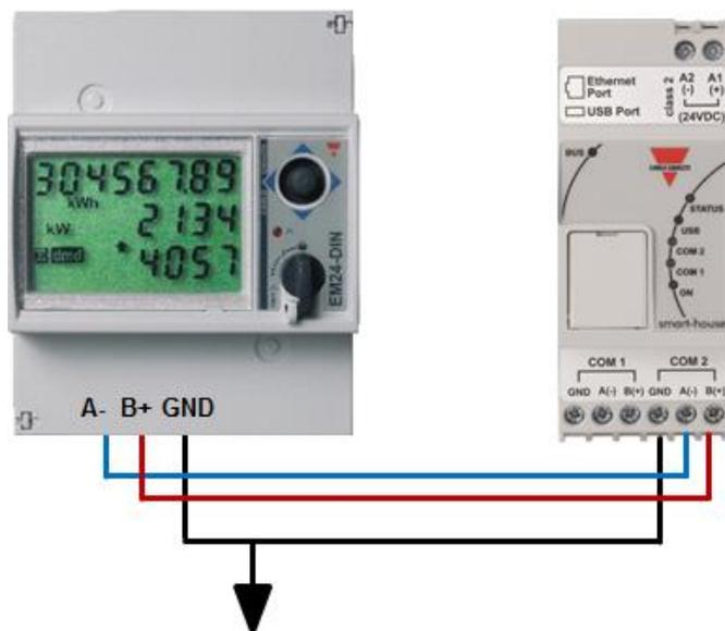
Different types of energy meter can be mixed, and they can also have different baud rate (see the Sx tool software manual for more details about how to configure the Sx2WEB24 to manage them).
