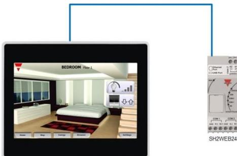
The TCP/IP device can be connected directly to the Sx2WEB24 with a peer to peer connection by using fixed IP (see the Sx tool manual to configure a fixed IP).
