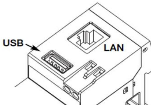
2. Insert the Pen-drive, making sure it is not write-protected and it is correctly formatted (FAT32).
