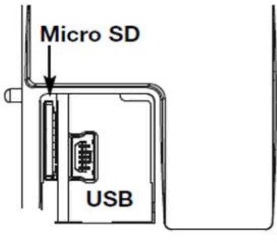
2. Insert the Micro SD card, making sure it is not write-protected and it is correctly formatted (FAT32).
