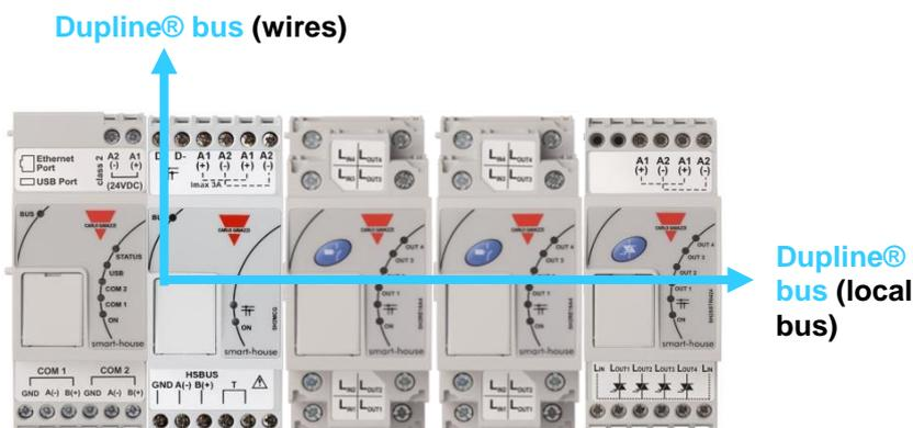
If more bus generators are connected in a DIN rail, they do not need to be plugged next to one other and they can also be mixed with the Dupline® I/O modules. The only rule that the installer has to take into account is that a Dupline® I/O module is connected to the Dupline® network generated by the last SH2MCG24 at its left. See picture below.
