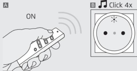
**Optional: Unpair the socket switch from a transmitter**
