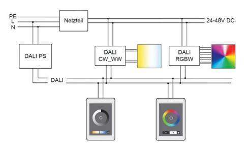
structure for the control of colour/colourtemperature
