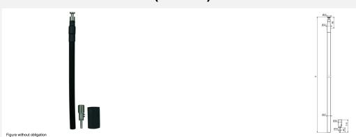
High-voltage-resistant, insulated down conductor for keeping the separation distance to electrically conductive parts according to IEC 62305-3.
