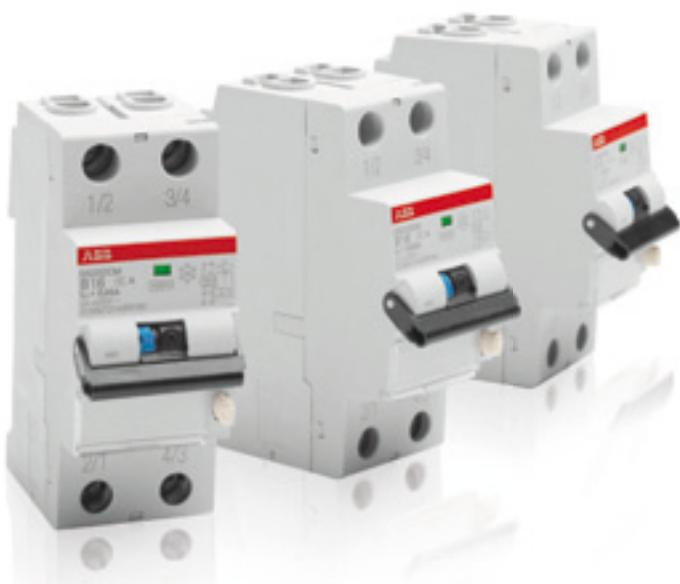
The DS201 series replaces the actual range of 1P+N RCBOs and combines protection against overcurrent and earth fault current in a single device. The range is available in three versions: DS201 L (with 4,5 kA breaking capacity), DS201 (with 6 kA breaking capacity) and DS201 M (with 10 kA breaking capacity), in compliance with the IEC/EN 61009 standard.
