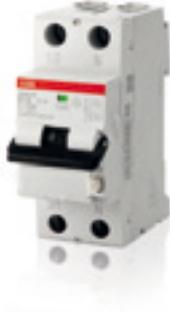
RCBO 1P+N, C characteristic, Icn=10 kA (acc. to IEC/EN 61009)
