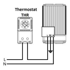
WARNING: FSHT is fitted with thermal cut out fuse in case of fan failure. It avoids temperature rises over value which could damage the unit.
