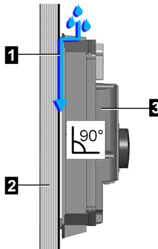
Fig. 6-11: Water drainage
