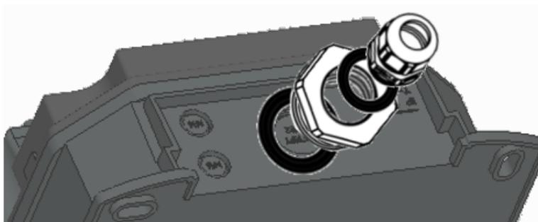
Fig. 7-17: Use of a reducing insert
