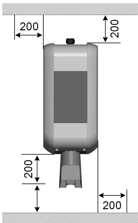
Fig. 6-12: Space requirement, specified in mm
