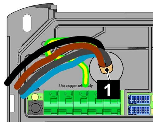
Double-membrane seals (flush-mounted cable installation)
