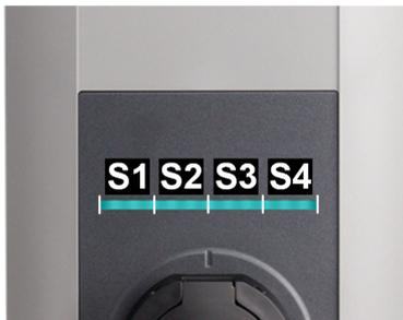
Fig. 5-9: Segments of the LED bar
