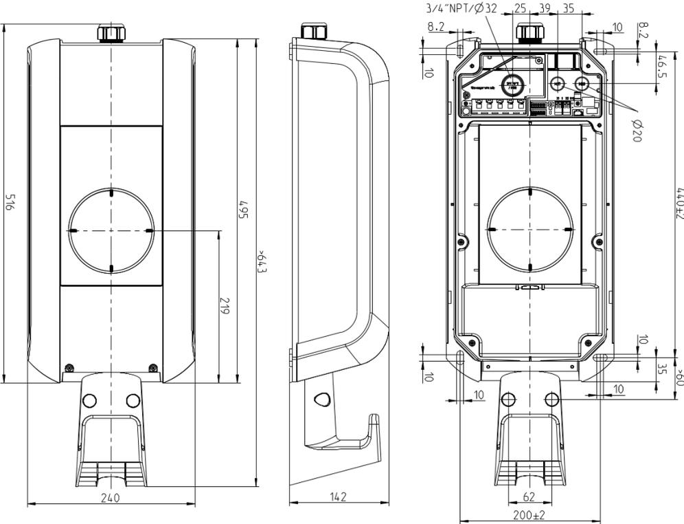
Fig. 12-23: Dimensions in millimeters
