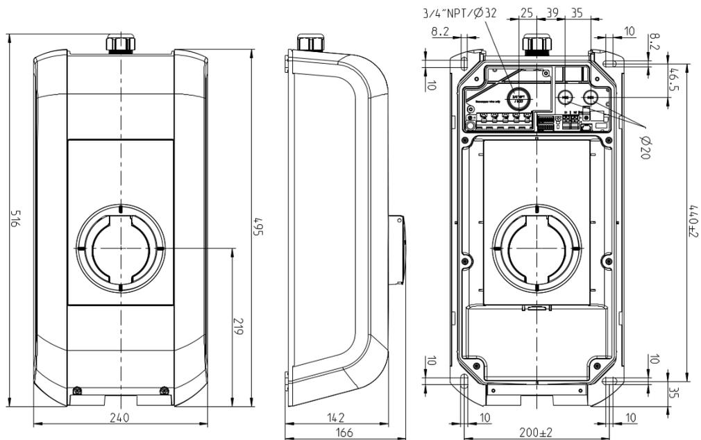
Fig. 12-22: Dimensions in millimeters
