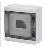
IP65 range of watertight anclosures from 4 to 72M with smoked transparent door. The main technical features are: reversible front and back panel, removable frames and panels with windows and detechable doors with up to 180° opening and lock accessory. The enclosures can be equipped with bipolar and unipolar terminal blocks, 80 A and 125 A, with screw wiring; they allow to create simple and neat wiring reducing the set-up time of the enclosure.
