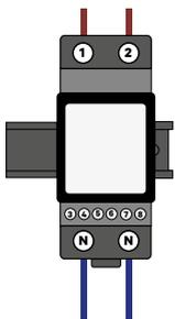
1. Install the power meter on the DIN rail.
