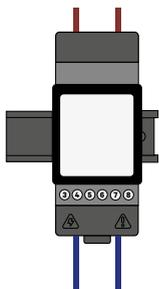
2. Install the phase and neutral. Verify that the phase and neutral are firmly anchored. Install the insulation plate on top of the screws.
