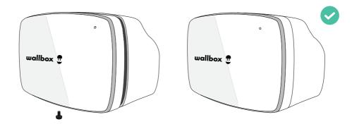
Recommended tightening torque 0.7 Nm +/- 10%
