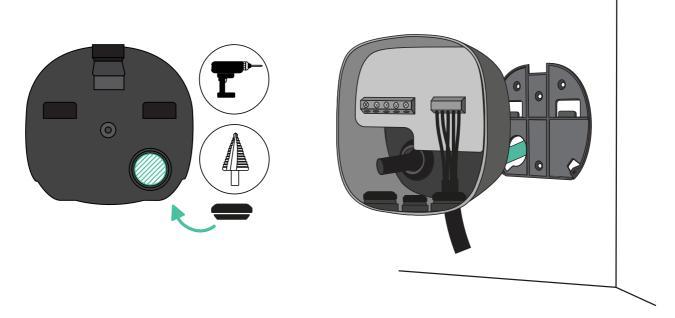
Fix your charger to the wall plate and then fix it using the appropriate screws.
