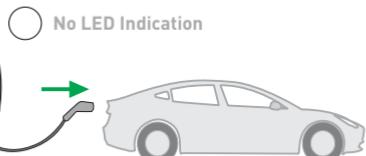
**2 - Insert the charging plug to the vehicle inlet.**
