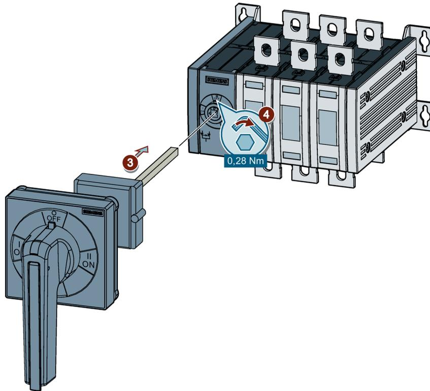
4. Fix the shaft to the door-coupling driver using a bolt.
