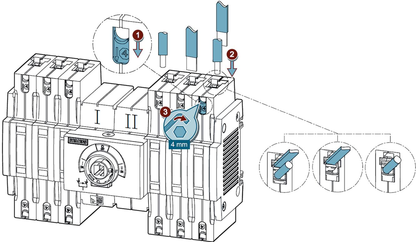
2. **If a flat cable is used:** Insert the cables into the lower openings of the box terminal.
