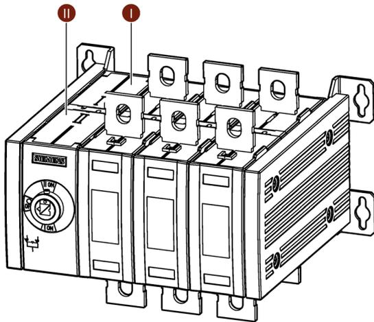
Switch I is at the rear and switch II is at the front with transfer switching equipment sizes 3, 4 and 5.
