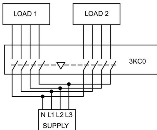
**Circuit diagram of 3KC0 as three-phase 4-wire network with three phases without neutral conductor (3PH)**
