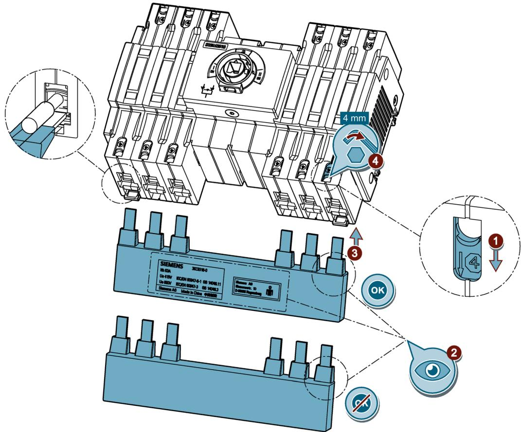
2. Ensure that the orientation of the bridging bar is correct.
