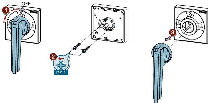
2. Loosen the bolts on the rear of the cover.
