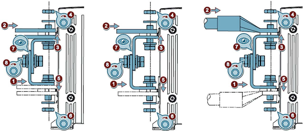
2. Position the first cable lug or first busbar at the connecting terminal.
