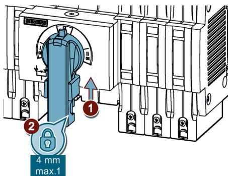
8.8.3.2 Padlocking mode of direct operating mechanism for size 3
