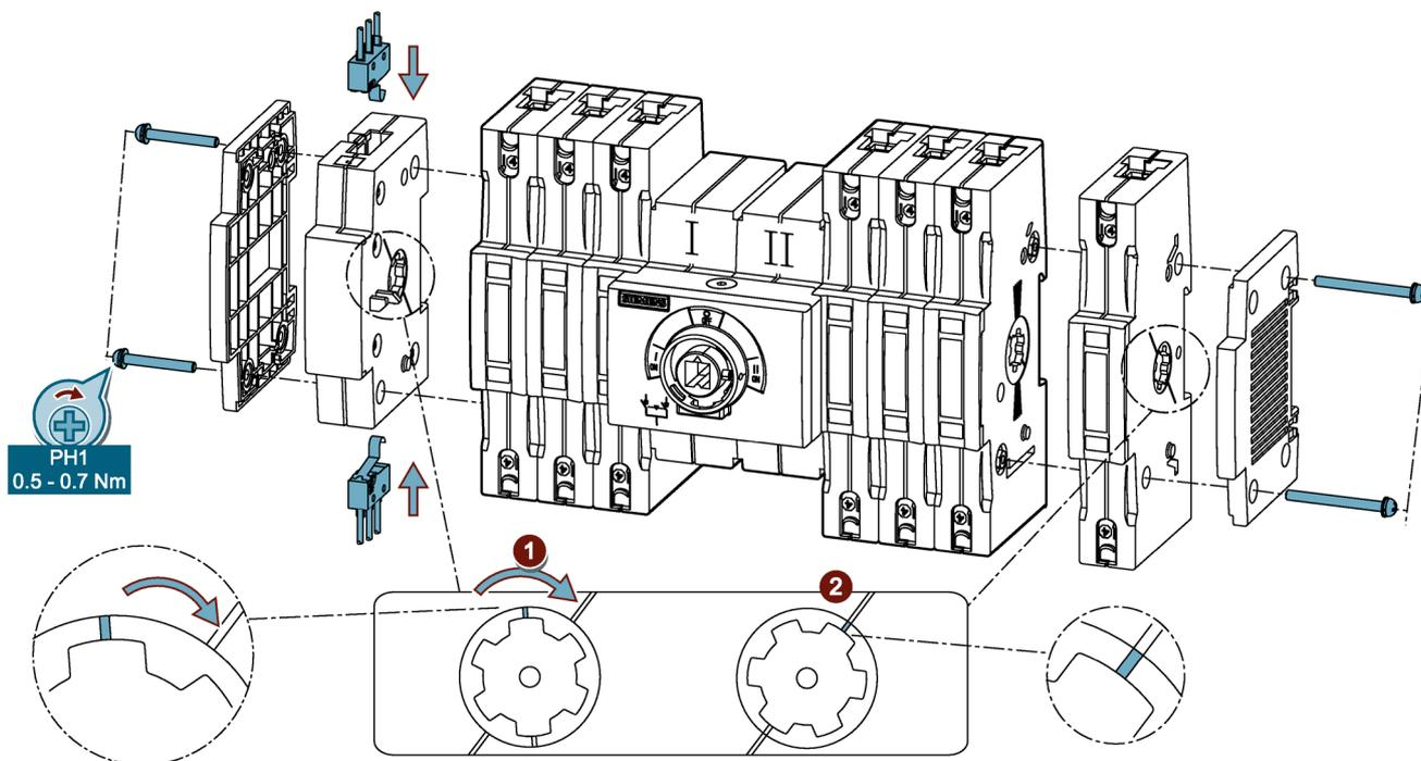
3. Mount the additional accessory on the transfer switching equipment (e.g. additional pole or auxiliary switch module).
