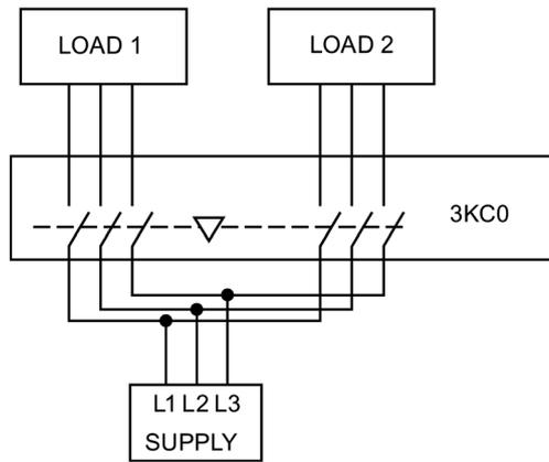
**Circuit diagram of 3KC0 as single-phase network with neutral conductor (1PH + N)**
