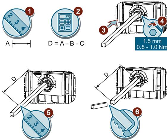
1. Measure clearance A from the mounting plate/rear panel of the control cabinet to the outside of the cabinet door. Observe the maximum values for A.
