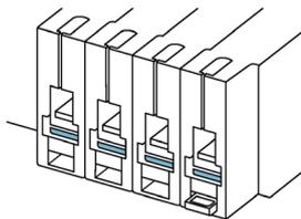
You can connect either the bridging bar accessory (3KC9118- or 3KC9218-) or a copper bar to the lower opening of the box terminal. You can find more information in chapter Connecting transfer switching equipment sizes 1 and 2 to the circuit (Page 41).
