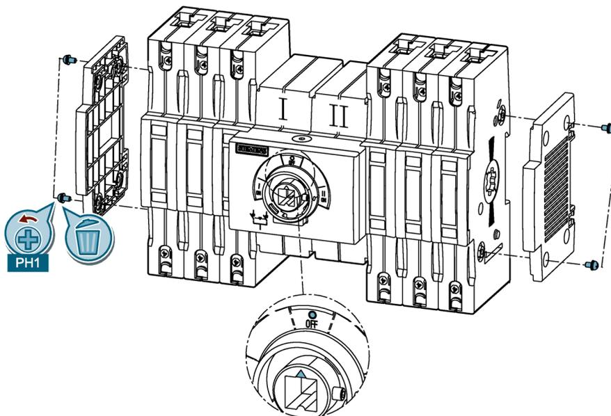
2. Rotate the shaft of the additional pole or auxiliary switch module to the correct position. Ensure that the pre-inscribed marks are aligned.
