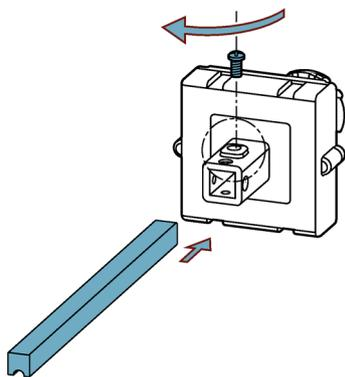
3. Insert the shaft into the 3KC0 until it engages.
