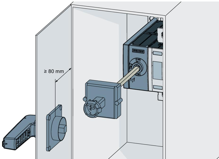
The clearance between the center hole in the cabinet door (shaft) and the hinge of the cabinet door must be at least 80 mm.
