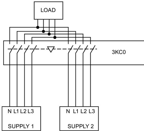
**Circuit diagram of 3KC0 as three-phase 4-wire network with three phases without neutral conductor (3PH)**
