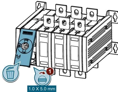
2. Mount the handle with the direct operating mechanism attached on the transfer switching equipment.
