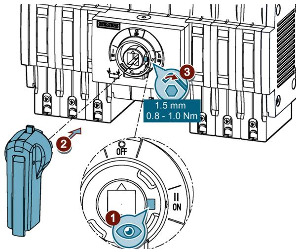
2. Loosen the bolt until the recess is completely free.
