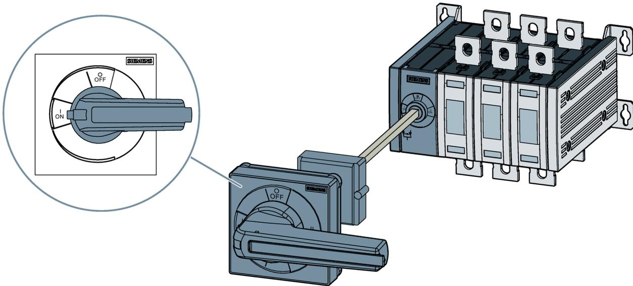
If the 3KC0 is rotated by 90° during mounting, the position of the 8UD1 handle is in the right-hand position. The tongue and groove connection on the coupling drivers and on the shaft coupling can be adjusted in steps of 90° in order to move it to the top position.
