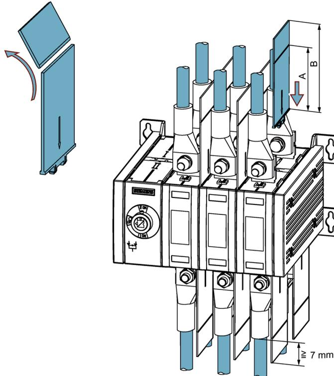
2. Insert the phase barrier into the appropriate mounting channel on the transfer switching equipment.
