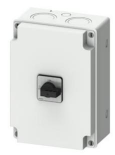
SENTRON switch disconnector 3LD in molded-plastic enclosure, repair and maintenance switch with EMC plate, 3-pole lu: 125A, AC23A 400V at 50/60Hz: 45kW, used with frequency converter: AC20 400V at 0-550Hz: 45kW, 1NO + 1NC 20-150ms leading, molded-plastic encapsulation for metric cable gland, knob-operated mechanism, black, lockable in 0- and I-position, incl. cable shield clamps and hose clamps
