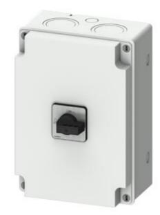
SENTRON switch disconnector 3LD in molded-plastic enclosure, repair and maintenance switch with EMC plate, 6-pole lu: 63A, AC23A 400V at 50/60Hz: 22kW, used with frequency converter: AC20 400V at 0-550Hz: 18,5kW, 1NO + 1NC 20-150ms leading, molded-plastic encapsulation for metric cable gland, knob-operated mechanism, black, lockable in 0- and I-position, incl. cable shield clamps and hose clamps
