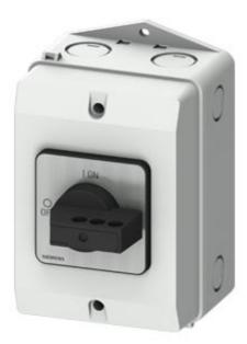
SENTRON switch disconnector 3LD in molded-plastic enclosure , repair and maintenance switch with EMC plate, 3-pole lu: 16A, AC23A 400V at 50/60Hz: 7,5kW, used with frequency converter: AC20 400V at 0-550Hz: 4kW, 1NO + 1NC 20-150ms leading, molded-plastic encapsulation for metric cable gland, knob-operated mechanism, black, lockable in 0- and I-position, incl. cable shield clamps
