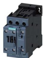
power contactor, AC-3e/AC-3, 12 A, 5.5 kW / 400 V, 3-pole, 24 V DC, auxiliary contacts: 1 NO + 1 NC, screw terminal
