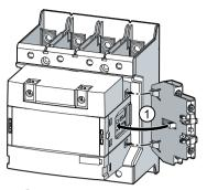
1 Attach the lateral auxiliary switch to the contactor and snap it on.
