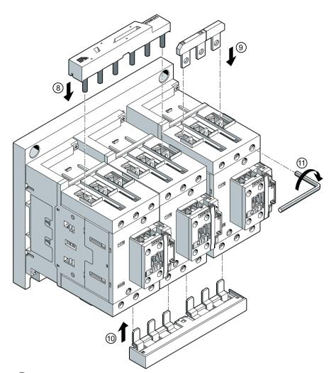
8 Attach the wiring module for connecting the main current paths to contactors Q11 and Q13 from above.
