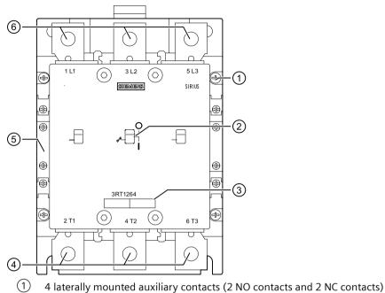
2 Contact erosion indicator and switch position indicator
