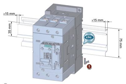
1 Position the device on the top edge of the mounting rail and press it down until it snaps onto the bottom edge of the rail.
