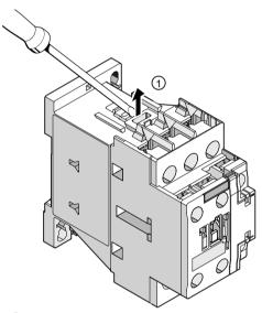
① Use a screwdriver to lift up the retaining clips between the rear and front halves of the contactor.
