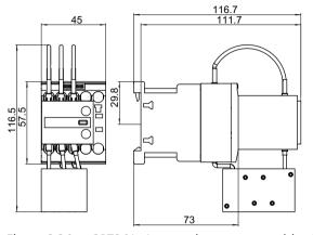
Figure C-36 3RT261.-1...capacitor contactors (size S00)
