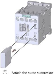
Attach the surge suppressor onto the front of the contactor. Codes help you to identify which is the correct way up when inserting the device. Note:
