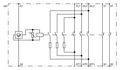
11.4 Reversing contactor assemblies (S00 / S0 / S2 / S3)
