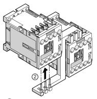
2 Attach the contactor onto the link module's pins from above.
