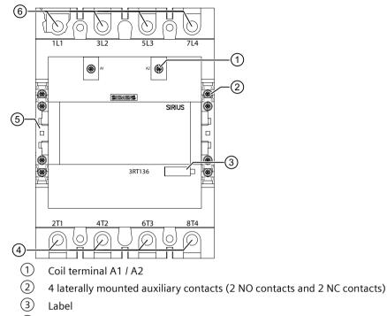
(4) Main circuit connection as busbar connection (T1, T2, T3, T4)
