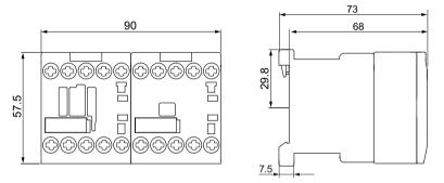
Figure C-9 Latched 4-pole contactor relay 3RH24..-1 (screw-type connection system)
