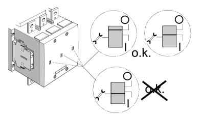
Figure 7-6 Contact erosion indicator and switch position indicator
