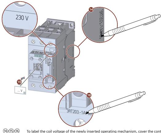
)/(15)/(16) To label the coil voltage of the newly inserted operating mechanism, cover the control supply voltage specification with the labels supplied. Thoroughly cross out the article number.
