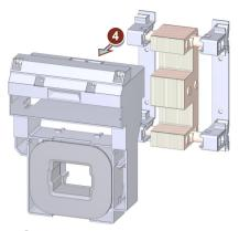
(4) Remove the solenoid coil.
