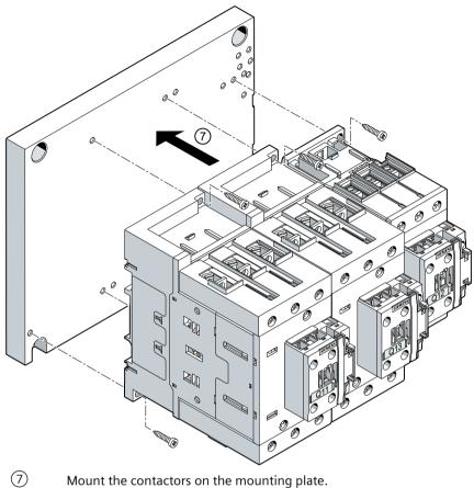
Mount the contactors on the mounting plate. Screws: 6 x M6 Tightening torque: 1.6 Nm
