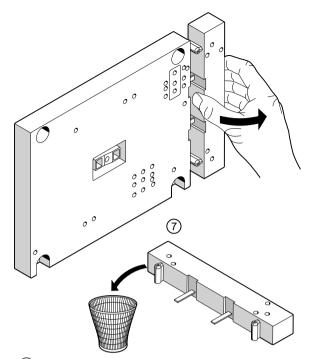
(7) When using the mounting plate (for S2 3RA2932-2F; for S3 3RA2942-2F), you must remove its side section.
