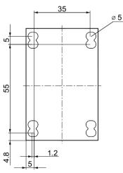
Figure C-13 Drilling plan for contactors and contactor relays with spring-loaded connections (size S00)
