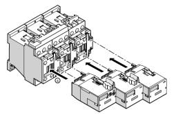
(4) Attach the basic module/coupling module to the contactor from the front. To do this, insert the contacts into the openings on the contactor.
