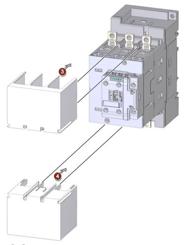
(3) (4) Slide the terminal cover for cable lug connection and busbar connection into the guide tabs provided for this on the contactor.
