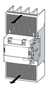
9.39 Terminal cover for 3RT135, 3RT136 and 3RT137 contactors (sizes S6 to S12)
