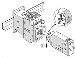
③ Snap the mechanical latch onto the center of the contactor until it engages.
