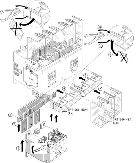
The diagram below uses the 3RT1.5 contactor size S6 as an example of mounting the 3RT1956-4EA4 terminal cover for cable lug connection and busbar connection.
