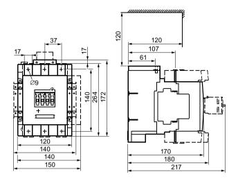
Drilling diagram for 3RT1.5. contactors
