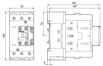
Figure C-34 3RT204.-3 (spring-loaded connection system)
