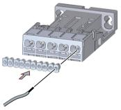
Figure 9-21 Insulating stop on spring-loaded connection
