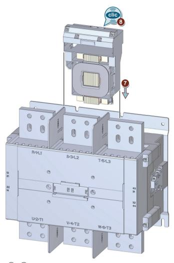
$\overline{(7)}$  / (8) Make sure that the solenoid coil clearly engages on reinsertion.
