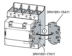
① Attach the second lateral auxiliary switch to the mounted lateral auxiliary switch and snap it on.
