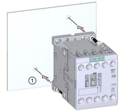
Using two M4 screws, plain washers and spring washers, screw the contactor tight into the designated drill holes diagonally. Maximum tightening torque 1.2 to 1.6 Nm
