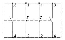
Auxiliary switch, for mounting on the front, 4-pole, 2 NO contacts, 2 NC contacts
