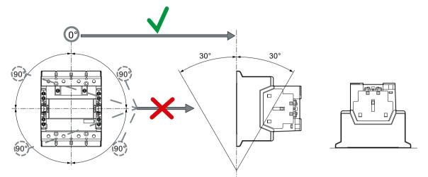
Figure 7-3 Mounting positions 3RT135, 3RT136 and 3RT137
