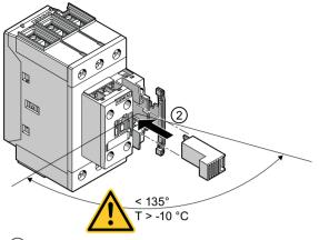
2 Insert the control kit into the opening until it engages.
