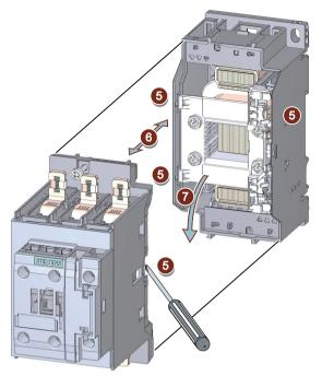
(5) (6) Push the two halves of the contactor apart. Note the lateral latching here. Take the solenoid coil out of the rear half of the contactor.
