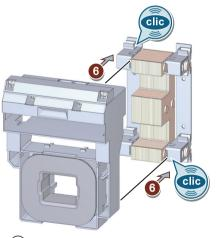
6 Slide the new solenoid coil onto the iron core.
