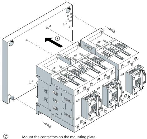
Mount the contactors on the mounting plate.
