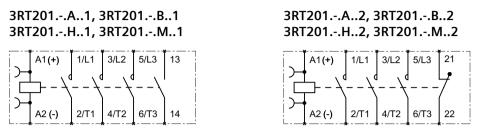
S00 contactor, without RC circuit, 1 NO contact S00 contactor, without RC circuit, 1 NC contact
