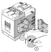
Mounting a second lateral auxiliary switch on 3RT1.5, 3RT1.6 and 3RT1.7 contactors
