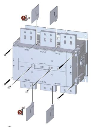
5 Slide the phase barriers into the openings provided on the contactor.
