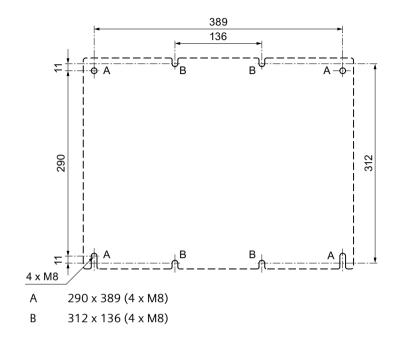
Drilling plan for 3RT1485 and 3RT1486 contactors
