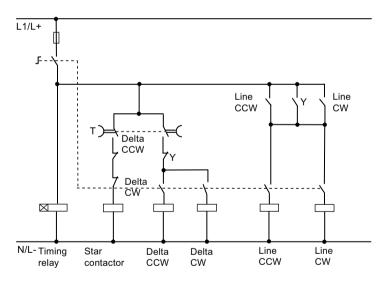
Figure 6-27 Control circuit of the contactor assembly for star-delta (wye-delta) start
