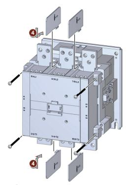
④ Slide the phase barriers into the openings provided on the contactor.
