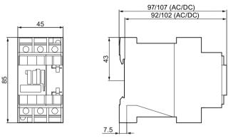
Figure C-20 3RT2.2.-4 contactors (ring cable lug connection system)
