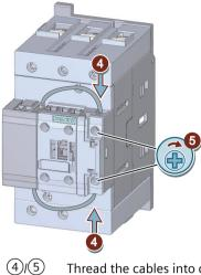
Thread the cables into coil terminals A1 and A2 of the contactor and screw them in place.
