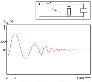
Figure 9-10 RC circuit with RC element (AC/DC operation)
