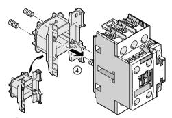
(4) Insert the new solenoid coil. In doing so, make sure that the springs between the solenoid coil and the front half of the contactor are properly located on the support.
