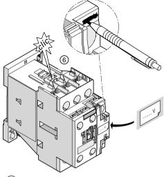
6 Write the coil voltage of the newly inserted operating mechanism onto the label supplied and stick the label onto the front panel of the contactor, as shown in the diagram. Thoroughly cross out the coil voltage stated above terminal A1.
