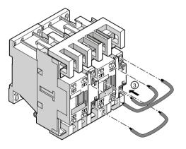
③ To connect the control current paths, strip the conductors and push them into the contactor terminals.
