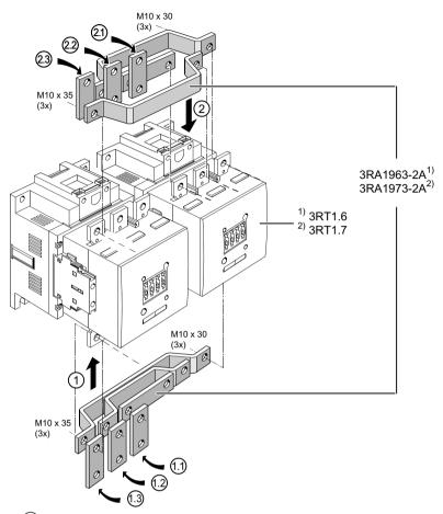
① Slide the wiring modules for connection without box terminal block onto the contactors from below.
