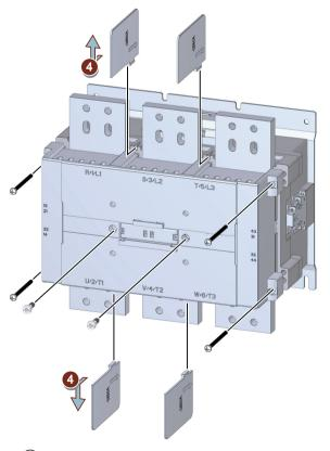
4 Pull the phase barriers forward slightly. Remove the phase barriers.
