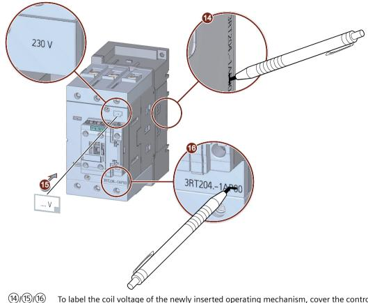
14)/(15)/(16) To label the coil voltage of the newly inserted operating mechanism, cover the control supply voltage specification with the labels supplied. Thoroughly cross out the article number.
