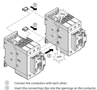
inservice connecting clips into the openings on the contactor.
