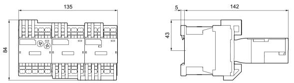
Figure C-61 3RA241.-8X.31-2 contactor assemblies for star-delta (wye-delta) start (size S00, spring-loaded connection system)
