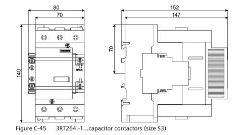
3RT264.-1...capacitor contactors (size S3)
