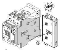
3 Attach the 4th pole to the other side of the same contactor by hooking it into the openings on the contactor and snapping the pole to the contactor.
