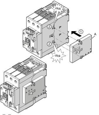
(1)/(2) Insert the mechanical interlock (3RA2934-2B) into the opening on the right-hand side of the contactor.
