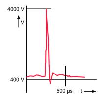
Figure 9-15 Counter-source voltage without RC circuit
