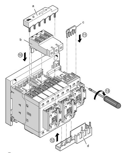
(1) Attach the wiring module for connecting the main current paths to contactors Q11 and Q13 from above (a).
