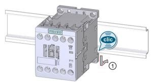
(1) Position the device on the top edge of the mounting rail and press it down until it snaps onto the bottom edge of the rail.
