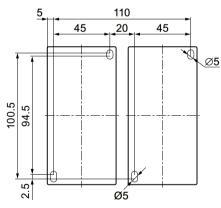
Figure C-58 Drilling diagram for 3RA233.-8XB30-1 reversing contactor assemblies
