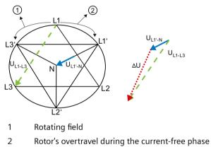
Figure 6-22 Phasor diagram for star-delta switchover during clockwise rotation with motor phases connected correctly
