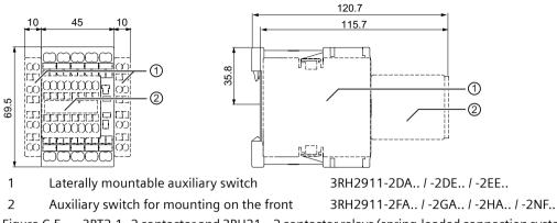
Figure C-5 3RT2.1.-2 contactor and 3RH21..-2 contactor relays (spring-loaded connection system) with auxiliary switches mounted
