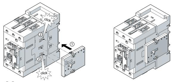
(1)/(2) Insert the mechanical interlock (3RA2934-2B) into the opening on the right-hand side of the contactor. Optional component A (mechanical interlock) is mandatory for mechanical interlocking.
