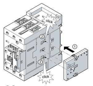
(1)/(2) Insert the mechanical interlock (3RA2934-2B) into the opening on the right-hand side of contactor Q13.
