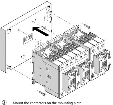
8) Mount the contactors on the mounting plate Screws: 6 x M6 Tightening torque: 1.6 Nm
