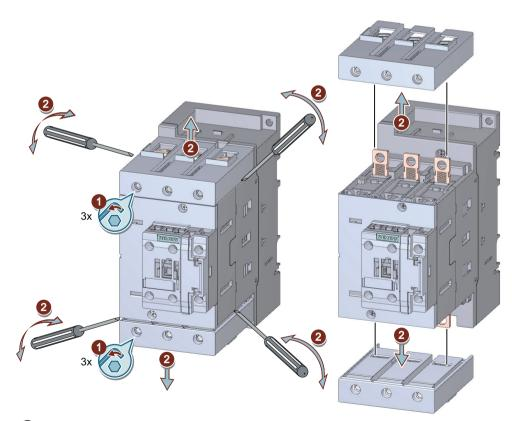
① Use an Allen key to undo the screws of the detachable box terminal block.
