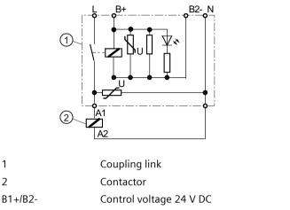
L1/N Rated control supply voltage for the selected contactor
