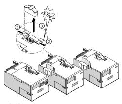
2/3 Remove the interface connection from the slot by lifting it up and out.
