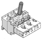
5 Push the locking slide down with a screwdriver until it engages.
