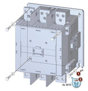
The following representations show the wall mounting options for the 3RT1485, 3RT1486 and 3RT1487 contactors.
