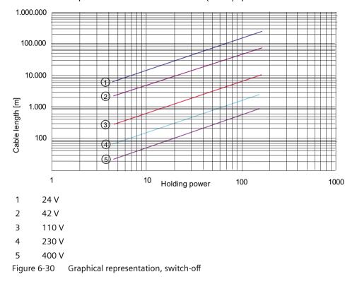
Maximum cable length [m] in the case of disconnection via pushbutton switch control on AC (50 Hz) operated contactors
