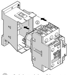
2 Push the two halves of the contactor apart.
