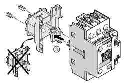
3 Take the solenoid coil out of the front half of the contactor.
