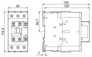
Figure C-28 3RT2.3.-3 contactor (spring-loaded connection system)
