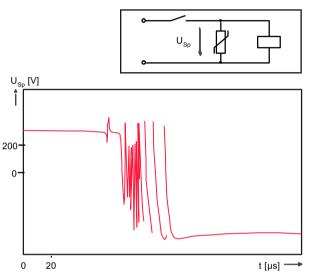
Figure 9-9 RC circuit with varistor (AC/DC operation)
