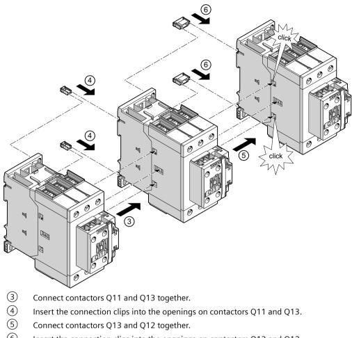
(6) Insert the connection clips into the openings on contactors Q13 and Q12.
