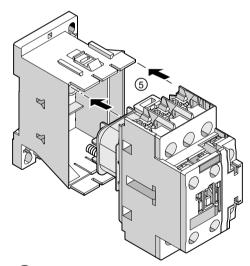
(5) Reattach the front part of the contactor onto the rear half until the retaining clips engage.
