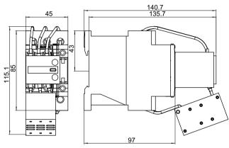
Figure C-38 3RT2625-1A... capacitor contactors (size S0)
