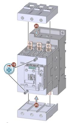
19 Tighten the screws to secure the cover (1.1 to 1.3 Nm).
