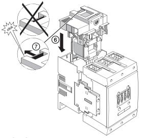
(6) (7) When re-installing, ensure that the interlock clearly engages again:
