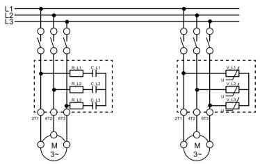
Figure 9-14 EMC suppression module, circuit diagram
