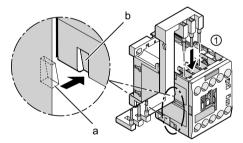
(1) Insert the pins of the link module into the contactor's terminal openings from above until they are securely in position. Make sure that the wedge (a) engages in the groove (b) provided on the contactor for this purpose.
