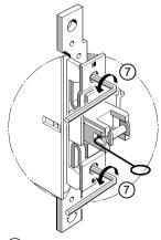
⑦ Undo the two screws that fix the non-movable contacts.
