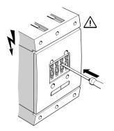
With 3RT105 / 3RT106 / 3RT107 / 3RT145 / 3RT146 / 3RT147 air-break contactors, the lateral auxiliary contacts can be operated for test purposes by pressing the auxiliary switch receptacle / switch position indicator on the front. By doing this the main contacts would also touch, without resulting in contact resilience.
