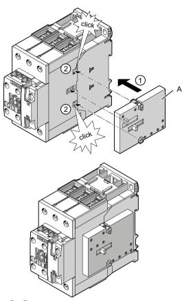
(1)/(2) Insert the mechanical interlock (3RA2934-2B) into the opening on the right-hand side of contactor Q13.
