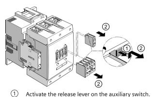
2 Push the auxiliary switch up and pull it forward to remove it from the contactor.
