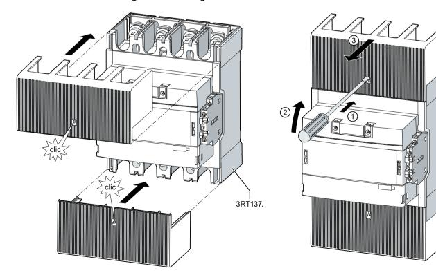
9.40 Mechanical interlock for 3RT135, 3RT136 and 3RT137 contactors (sizes S6 to S12)
