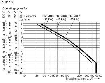
The contact service life is essentially dependent on the breaking current. The characteristic curves apply to:
