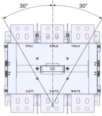
Figure 7-5 Mounting position 3RT148.
