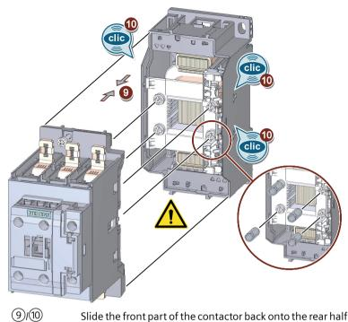
Slide the front part of the contactor back onto the rear half until the retaining clips engage. In doing so, make sure that the springs between the solenoid coil and the front half of the contactor are properly located on the support.
