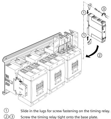
Screw the timing relay tight onto the base plate.
