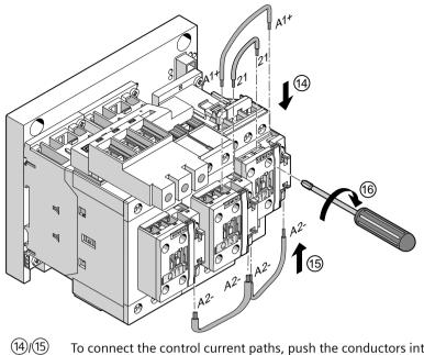
To connect the control current paths, push the conductors into the contactor terminals. To connect the coil contacts, push the conductors into the contactor terminals.
