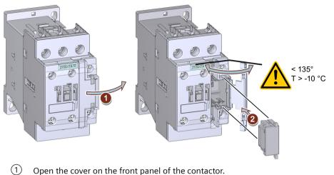
Insert the surge suppressor into the opening until it engages. Close the cover on the front panel of the contactor.
