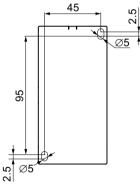
Figure C-44 Drilling diagram for 3RT263.-1.... capacitor contactors (size S2)
