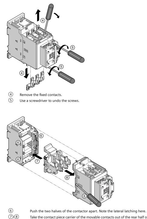
Take the contact piece carrier of the movable contacts out of the rear half of the contactor.
