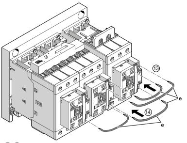
(13)/(14) To connect the control current paths, push the conductor (e) into the contactor terminals. To connect the coil contacts, push the conductors (e) into the contactor terminals.
