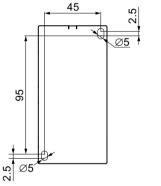
Figure C-30 Drilling plan for 3RT2.3. contactors (size S2)
