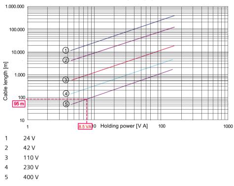
Figure 6-31 Graphical representation, switch-off - Example
