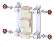
5 Slide both supports for the iron core together.
