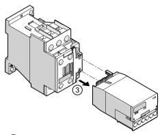
③ Pull the coupling module with the integrated mounting pins towards you off the coil terminal module.
