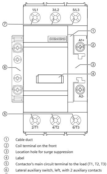
⑦ Contactor's main circuit terminal to the power network (L1, L2, L3)
