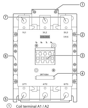
With an solid-state operating mechanism, additional terminals + / - 24 V DC signal (control via control input)
