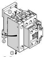
1/2 Remove the 4th pole from one of the two contactors by releasing the snap hooks.
