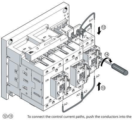
To connect the control current paths, push the conductors into the contactor terminals. To connect the coil contacts, push the conductors into the contactor terminals.
