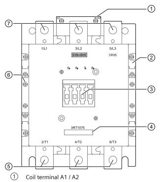
With an solid-state operating mechanism, additional terminals + / - 24 V DC signal (control via control input)
