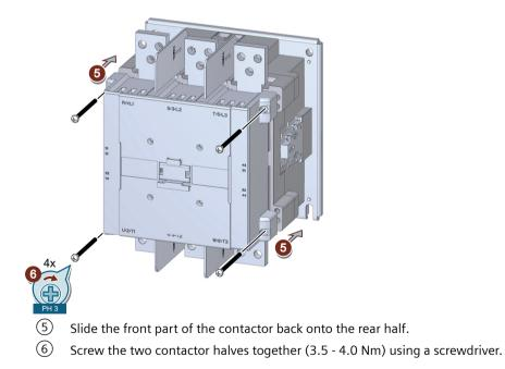
The following figures show examples of how to mount the 3RT1987-4AA1 phase barrier on the 3RT1487 contactors.
