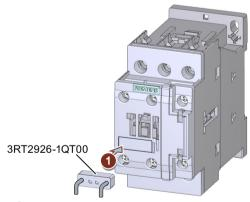
(1) Snap the LED display indicator module into the corresponding location hole provided on the front of the contactor.
