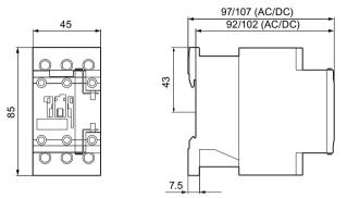
Figure C-14 3RT2.2.-1 contactors (screw-type connection system)
