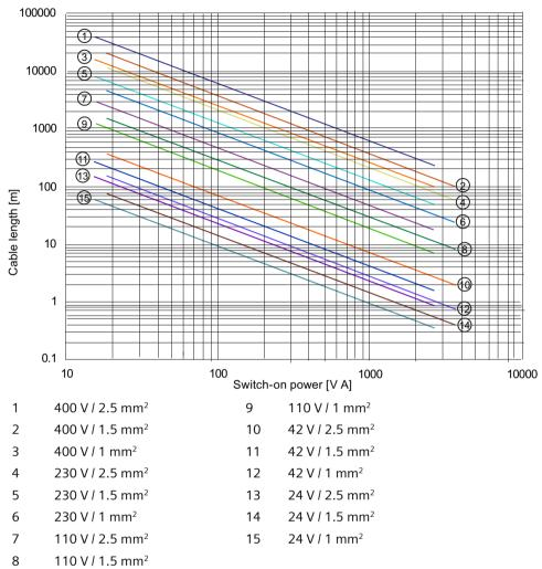
Maximum cable length with activation of AC (50 Hz) operated contactors
