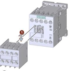
1 Push the auxiliary switch, which can be mounted on the front, into the location hole on the contactor. Pull it down until it engages.
