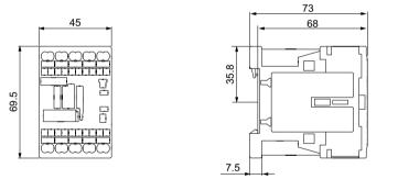
Figure C-4 3RT2.1.-2 contactor and 3RH21..-2 contactor relays (spring-loaded connection system)
