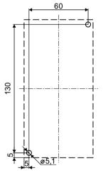
Figure C-46 Drilling diagram for 3RT264.-1.... capacitor contactors (size S3)
