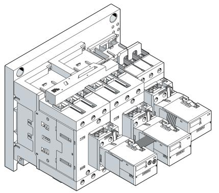
Figure 4-34**3RA24 contactor assembly for star-delta (wye-delta) start, screw connection, size S3 /**<br/>S3 / S2 (3RA2444-8X.32-1..., 3RA2445-8X.32-1..., 3RA2446-8X.32-1...)
