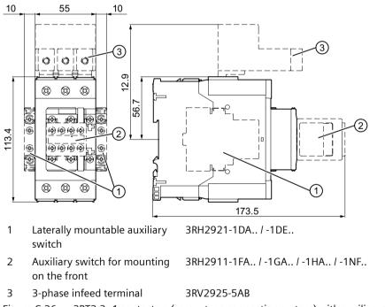
Figure C-26 3RT2.3.-1 contactors (screw-type connection system) with auxiliary switches mounted and 3-phase infeed terminal
