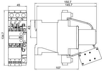
Figure C-40 3RT2628-1A... capacitor contactors (size S0)
