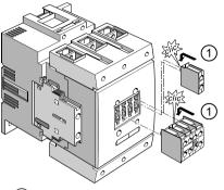
(1) Push the auxiliary switch, which can be mounted on the front, into the location hole on the contactor. Pull it down until it engages.
