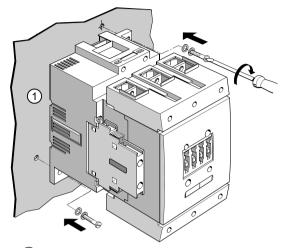
① Screw the contactor tight diagonally into the openings provided using two screws (size S6), plain washers and spring washers.
