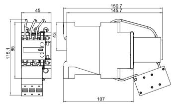
Figure C-39 3RT2625-1B... capacitor contactors (size S0)
