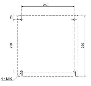
Drilling plan for 3RT1481 and 3RT1482 contactors
