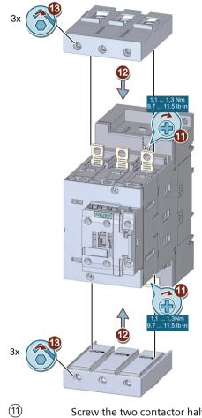
(11) (12)(13) Screw the two contactor halves together (1.1 - 1.3 Nm). Place the terminals on the device and push them towards the rear. Make sure the terminals engage.
