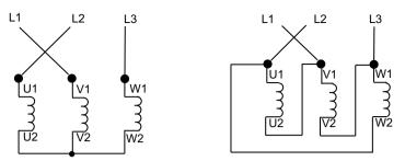
Figure 6-25 Correct connection of motor phases for counterclockwise motor rotation
