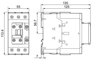
Figure C-25 3RT2.3.-1 contactor (screw-type connection system)
