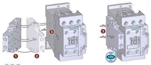
(1/2)/(3) Attach the lateral auxiliary switch to the contactor and snap it on.
