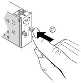
2 To deactivate it, press the right plunger. It can only be unlocked if the contactor coil is not excited.
