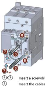
Insert a screwdriver into the spring-loaded connections and release them. Insert the cables into the spring-loaded terminals.
