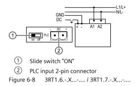
The contactor can be operated direct via an output of a controller (PLC).
