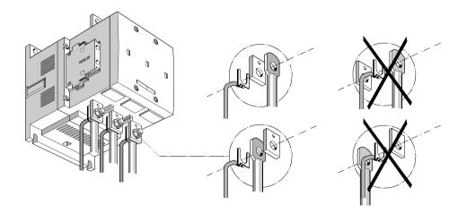
9.35 Main current path surge attenuation module for vacuum contactors
