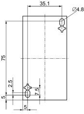
Figure C-22 Drilling plan for the 3RT202.-1 / 3RT232.-1 / 3RT252.-1 contactors (size S0)
