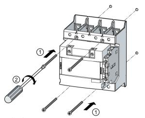
(1) (2) Screw the contactor tight into the openings provided using four screws.
