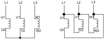
Figure 6-21 Correct connection of motor phases for clockwise rotation
