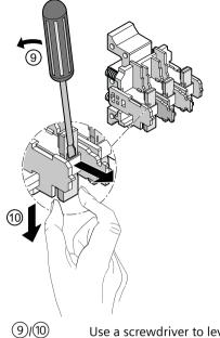
Use a screwdriver to lever the fixed contacts from the contact piece carrier.
