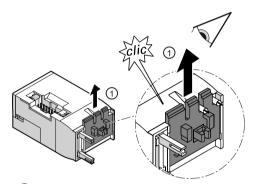
① Check that the locking slide is engaged in the topmost position.
