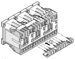
3 Attach the wiring module for connecting the main current paths to contactors Q13 and Q12 from below.
