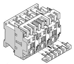
3 Attach the wiring modules for connecting the main current paths to contactors Q13 and Q12 from below.
