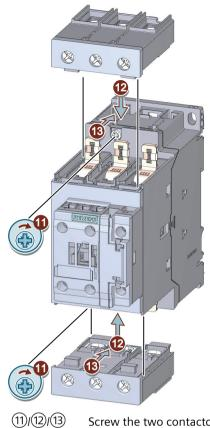
Screw the two contactor halves together (1.1 - 1.3 Nm). Place the terminals on the device and push them towards the rear. Make sure the terminals engage.
