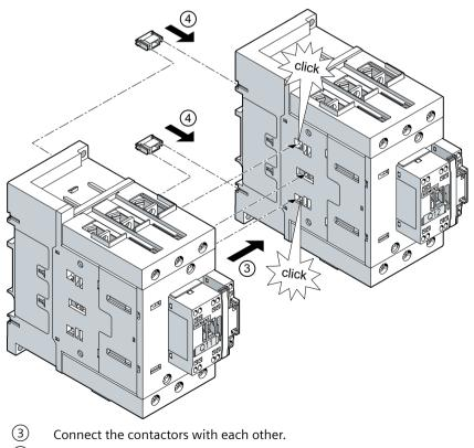
(4) Insert the connecting clips into the openings on the contactor.
