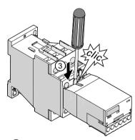
③ Use a screwdriver to press down the cover of the coupling module until it engages.
