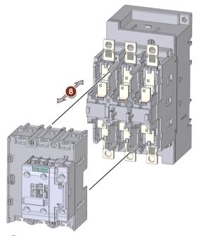
8 Take the contact piece carrier of the movable contacts out of the rear half of the contactor.
