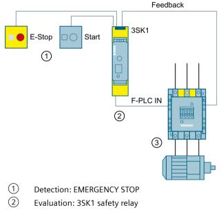
③ Reaction: 3RT1 contactor with fail-safe control input
