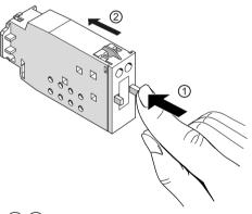
(1)/2 When snapping on, the switch position indicator's rod must be unlocked. Unlock the rod by pressing on the switch position indicator and pushing the rod into the mechanical latch as far as it will go.
