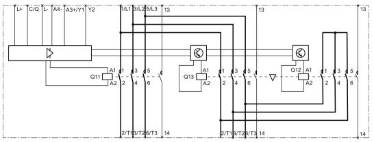
Figure 11-8 S00 contactor assembly for star-delta (wye-delta) start, with mounted function modules for IO-Link
