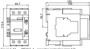
Figure C-43 3RT263.-1...capacitor contactors (size S2)
