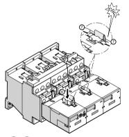
(6)/(7) Insert the coded module connector into the slot in the correct position from above until the module connector engages in the locking mechanism.
