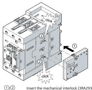
Insert the mechanical interlock (3RA2934-2B) into the opening on the right-hand side of contactor Q13.
