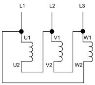
Figure 6-23 Motor phases connected incorrectly results in clockwise rotation
