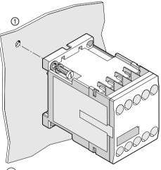
① Using two M4 screws (maximum tightening torque 1.2 to 1.6 Nm), plain washers, and spring washers, screw the OFF-delay device tight into the designated drill holes diagonally.
