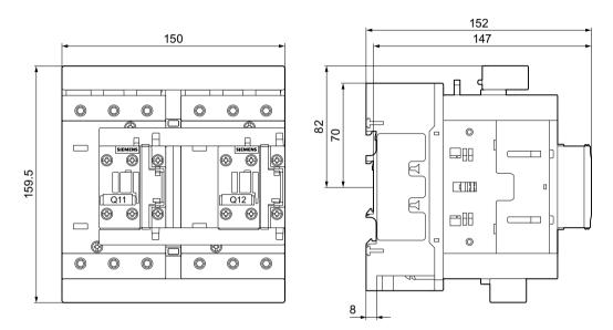
C.16.4.2 Drilling diagram for 3RA234.-8X.30-1 reversing contactor assemblies (size S3)
