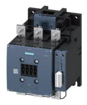
power contactor AC-1 400 A / 690 V / 40  $^{\circ}$ C 3-pole, Uc: 200-277 V AC(50-60 Hz) / DC PLC input 24 V DC drive: electronic auxiliary contacts 2 NO + 2 NC main circuit: busbar control and auxiliary circuit: screw terminal with remaining lifetime indicator
