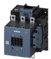
power contactor AC-1 275 A / 690 V / 40 °C 3-pole, Uc: 200-277 V AC(50-60 Hz) / DC PLC input 24 V DC drive: electronic auxiliary contacts 2 NO + 2 NC main circuit: busbar control and auxiliary circuit: screw terminal
