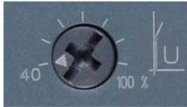
The starting voltage value is set with the U potentiometer. This value determines the starting torque of the motor. A lower starting voltage results in a lower starting torque (softer start) and a lower starting current.
