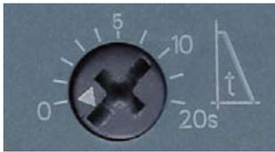
You can set a ramp-down time with the t potentiometer. This determines how long power should still be supplied to the motor after the ON command is removed. The torque generated in the motor is reduced by means of a voltage ramp function within this ramp-down time and the application stops smoothly.
