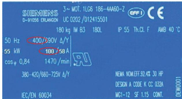
The rated operational current of the motor must be set with the  $I_e$  potentiometer according to the mains voltage and the motor connection (wye-delta). The electronic motor overload protection also refers to this set value if it is active. For the permissible settings referred to the required motor overload trip class, refer to chapter Motor current settings (Page 126).
