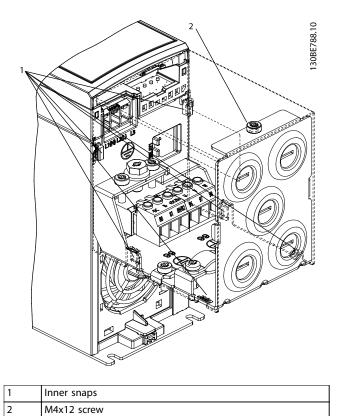
Illustration 1.6 Mounting the Base Cover, K1/K2/K3
