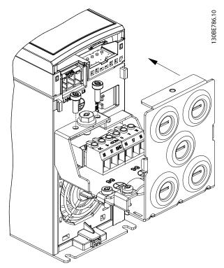
Illustration 1.4 Mounting the NEMA Bracket Plate, K1/K2/K3
