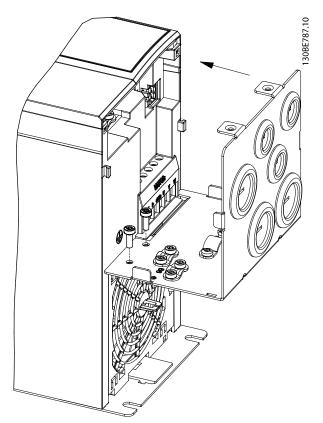
Illustration 1.5 Mounting the NEMA Bracket Plate, K4/K5
